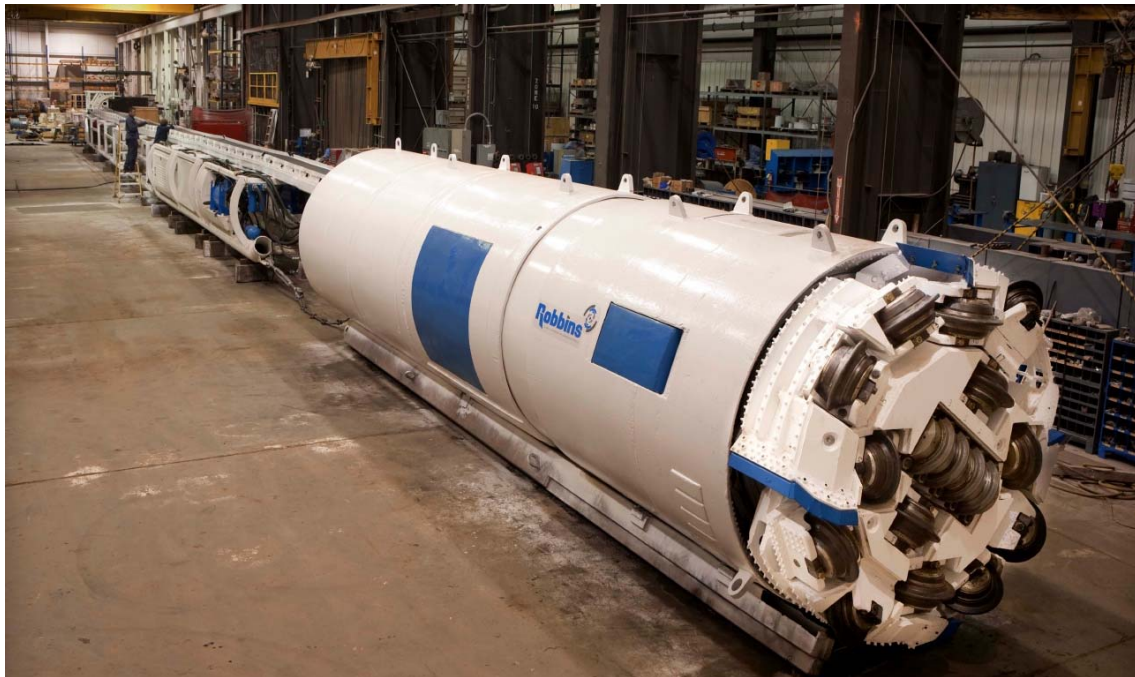
Figure 35: Tunnel Boring Machine (TBM)
