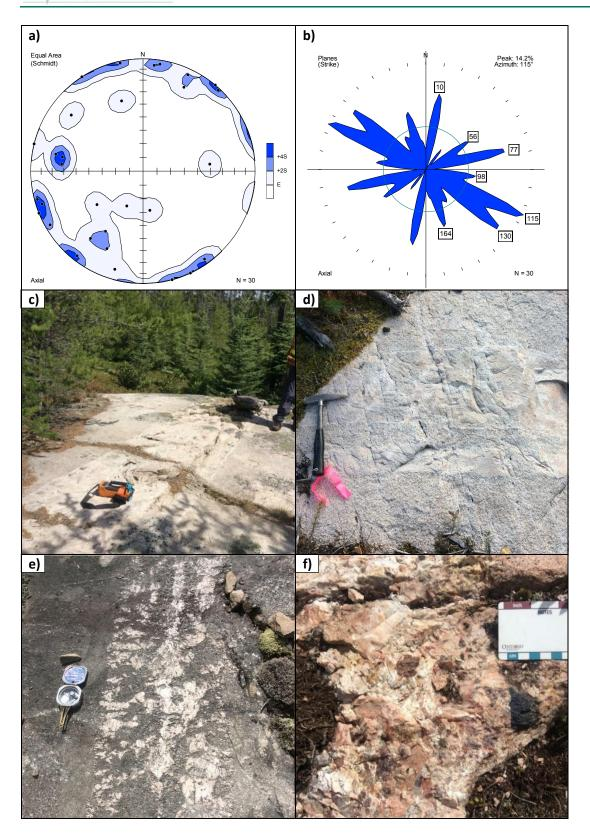
Figure 5.4.6: IGNACE AREA – Felsic Dykes Orientation Data and Field Examples
