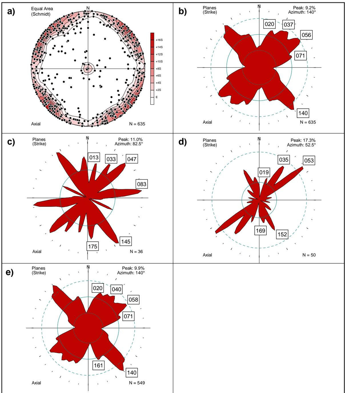
**Figure 5.2.11: Black-Pic Batholith Area – Joint Orientation Data**
