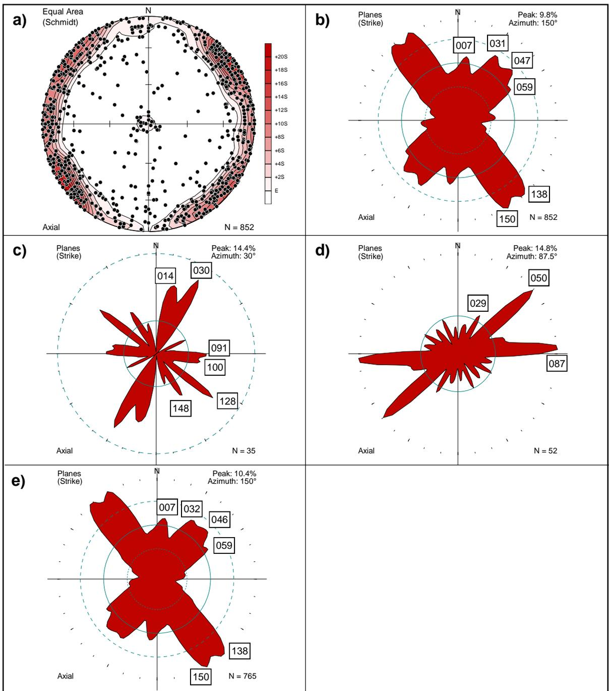
**Figure 5.1.15: Quetico Area – Joint Orientation Data**
