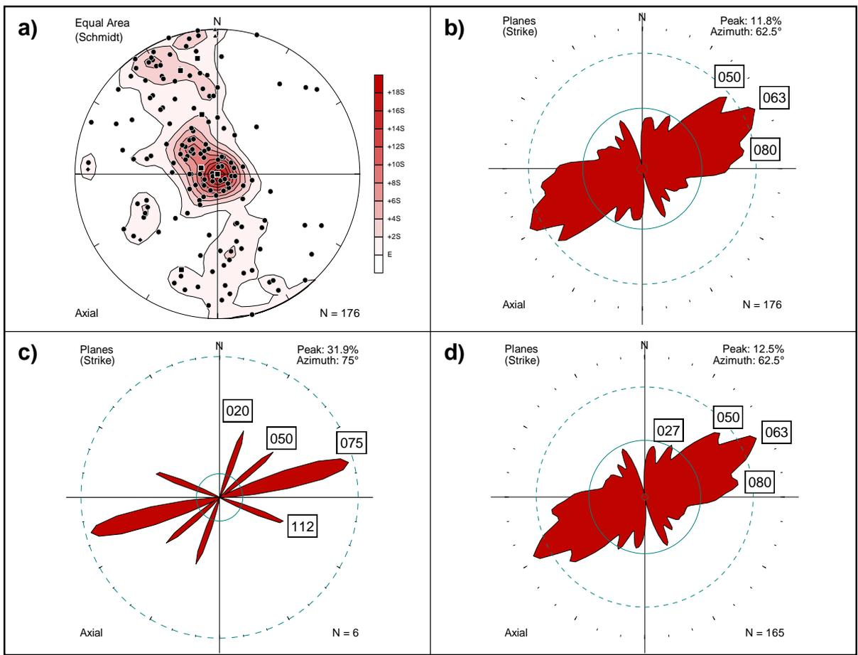
**Figure 5.2.8: Black-Pic Batholith Area – Foliation and Lineation Orientation Data**
