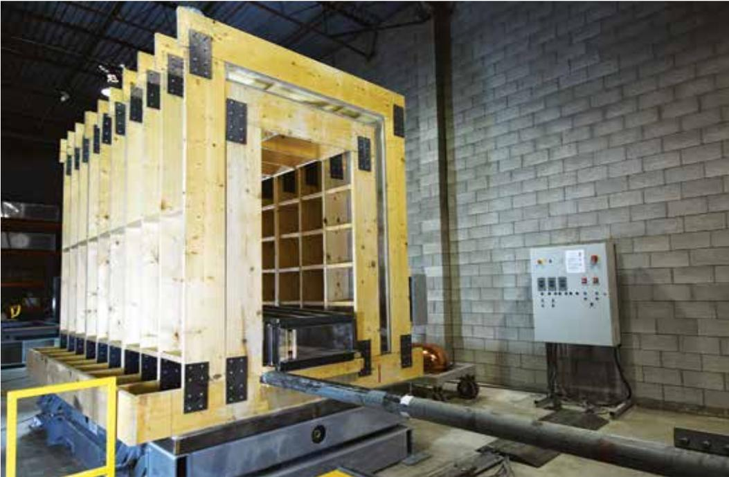
Bottom: This structure, designed by NWMO engineers, is used to test whether gapfill has completely filled the space between a buffer box and the excavated rock wall.
