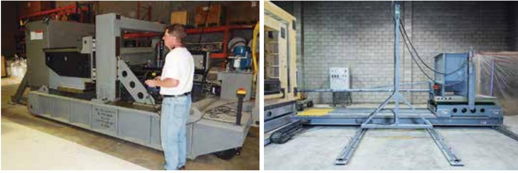
Top left: This prototype slip skid, designed by NWMO engineers, is designed to lift, transfer, and emplace the buffer box assembly onto a floor, as well as to stack buffer boxes.
