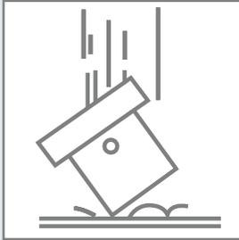
The package is dropped from nine metres (30 feet) onto a flat, unyielding surface (such as a steel-reinforced concrete pad), striking the surface in the orientation that will result in the most damage to the package.
