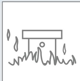
The same package used in the drop and puncture tests is then subjected to a fully engulfing petroleum fire. The fire temperature must reach 800 degrees Celsius (1,475 degrees Fahrenheit) for 30 minutes.
