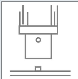
After the drop test, the same package is subjected to a one-metre (40-inch) free drop onto a 15-centimetre (six-inch) diameter steel bar at least 20 centimetres (eight inches) long.
