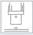
After the drop test, the same package is subjected to a one-metre (40-inch) free drop onto a 15-centimetre (six-inch) diameter steel bar at least 20 centimetres (eight inches) long. While the free-drop test simulates an impact that is spread over a larger area, this test looks at what would happen in a collision with a sharp object. The test demonstrates that the container will not puncture.
