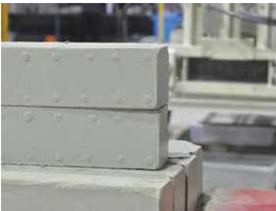
Bentonite bricks manufactured in Oakville, Ontario
