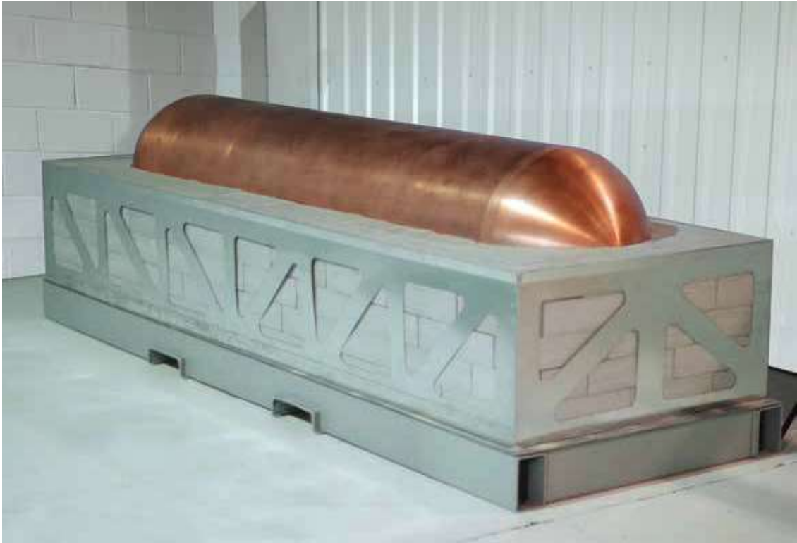
Fully assembled container placed in bentonite buffer box.
