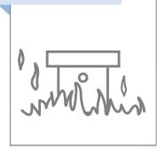
Using either computer analysis or physical testing methods, the same package used in the drop and puncture tests is then subjected to a fully engulfing petroleum fire. The fire temperature must reach 800 degrees Celsius (1,475 degrees Fahrenheit) for 30 minutes.
