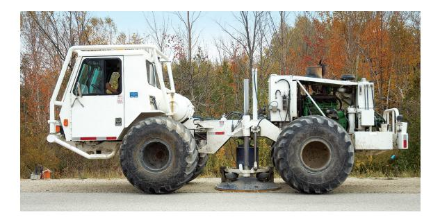
Vibroseis trucks are used to conduct 2-D seismic surveys.
