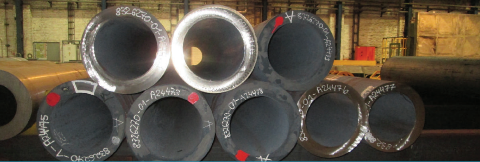
Raw pipes that will be used for 2019 serial manufacturing of the used fuel container.
