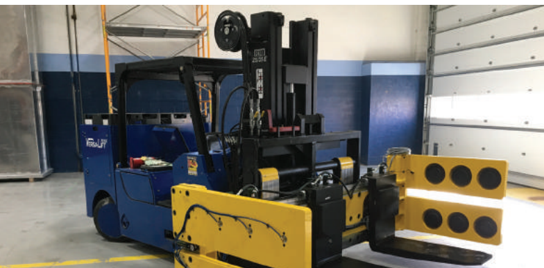
This specialized machine is designed for the emplacement of bentonite buffer boxes into emplacement rooms.
