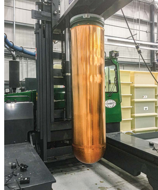
These pictures show advances to the copper-coating plating technology: The Nanovate™ Tank Plating System and supporting systems (left), and a prototype copper-coated container component produced in the plating system (right).
