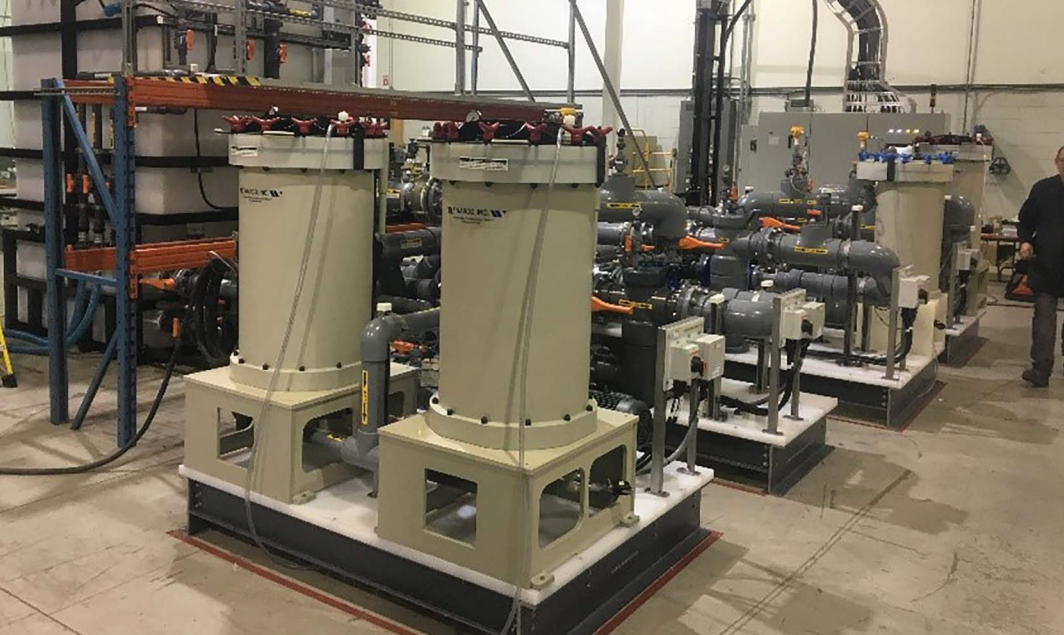
These pictures show advances to the copper-coating plating technology: The Nanovate™ Tank Plating System and supporting systems (left), and a prototype copper-coated container component produced in the plating system (right).
