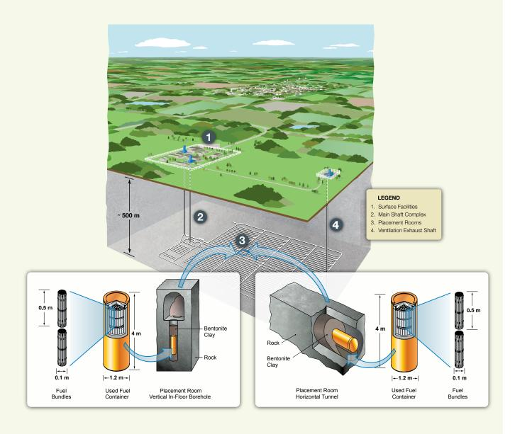
The containers will be placed in vertical boreholes drilled in the floor along the axis of a placement room, or placed horizontally within the confines of a placement room, depending on the nature of the rock and characteristics of the site.
