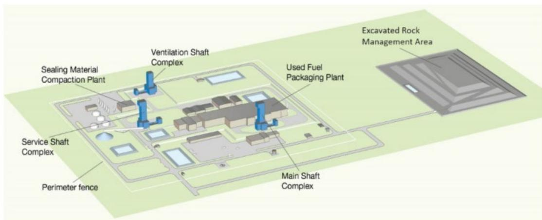
Figure 4-1: DGR Main Surface Facilities (NWMO, 2021b)
