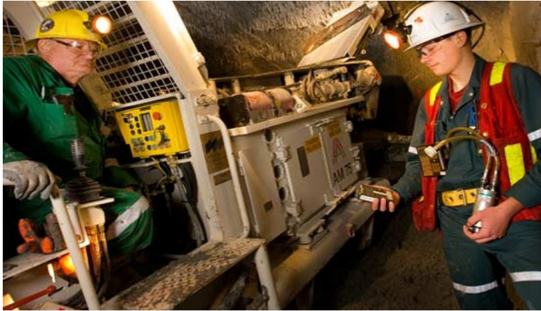
Figure 62: Manual Air Quality Monitoring
