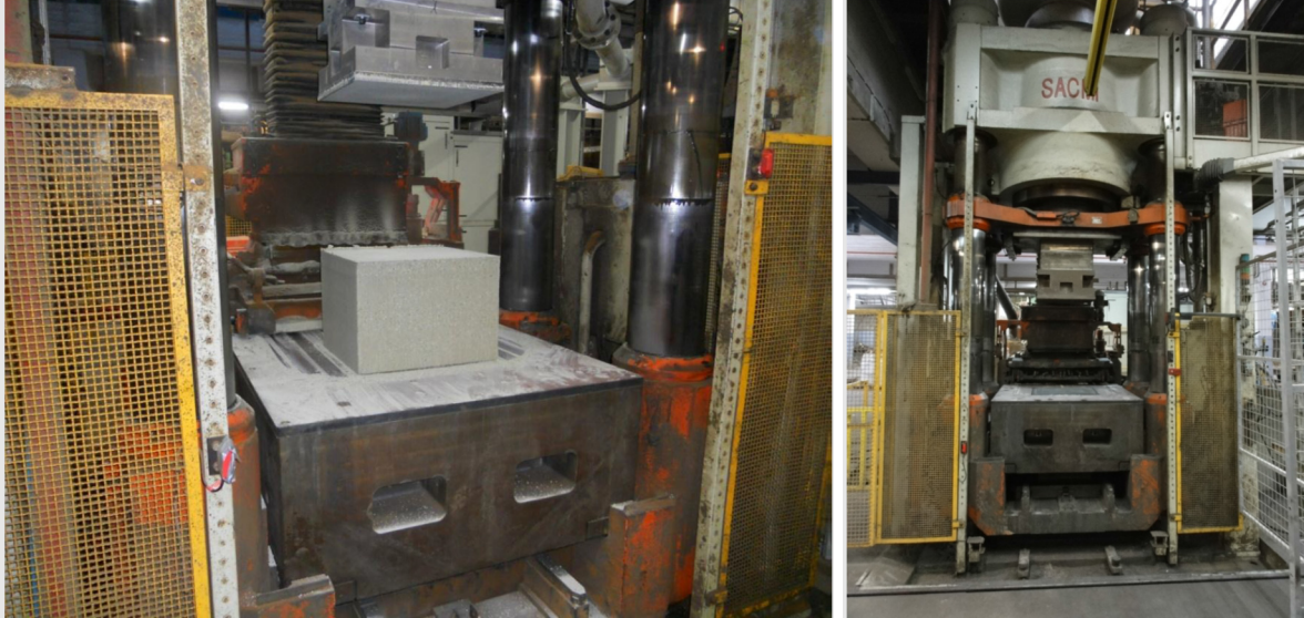
Figure 23: Example of Closed-Die Compaction Press
