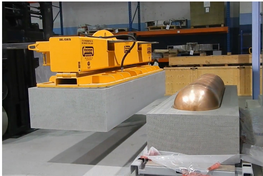
Figure 26: Prototype Buffer Block Vacuum Lift
