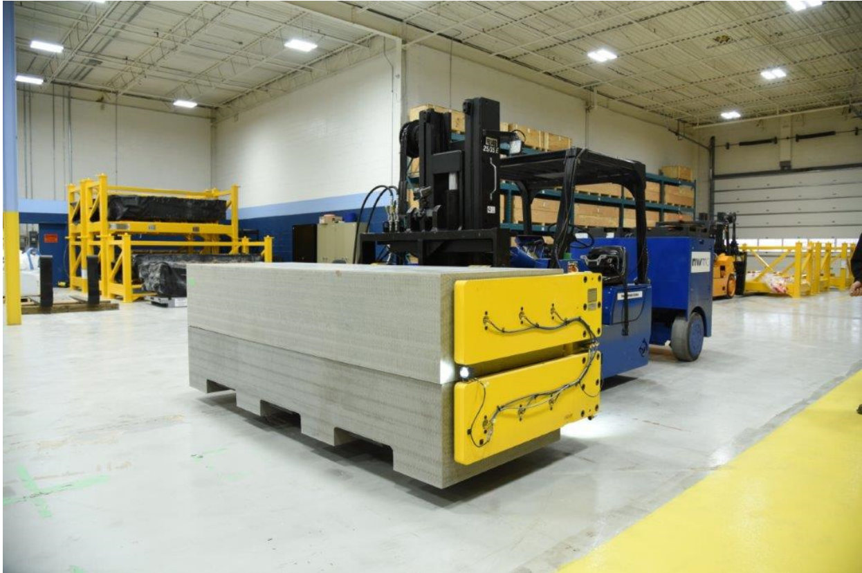
Figure 43: Prototype Buffer Box Emplacement Equipment
