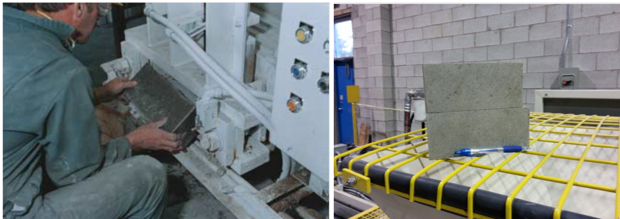
Figure 24: Portable Uniaxial Highly Compacted Bentonite (HCB) Brick Maker
