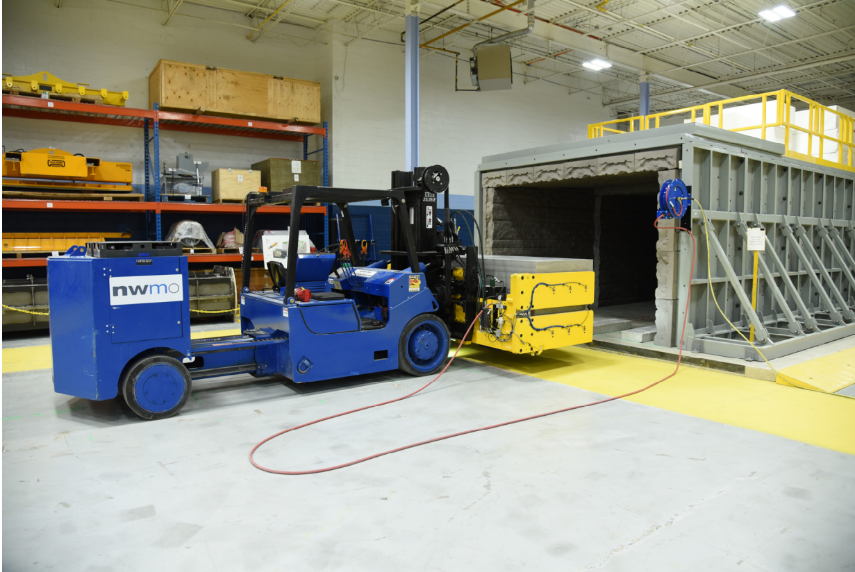
Figure 44: Prototype Emplacement Equipment entering the Mock-up Full-scale Emplacement Room
