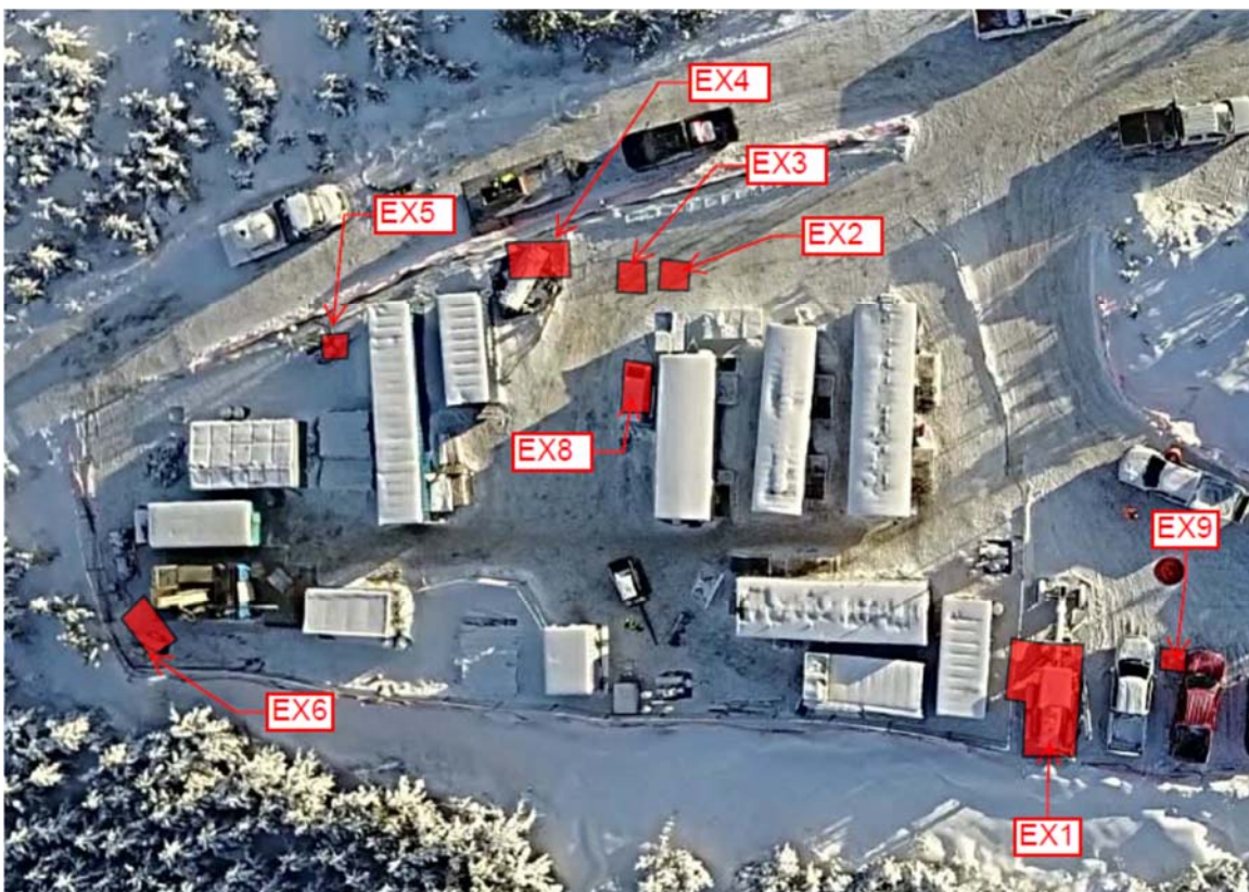
Figure 2: Location of the areas at the IG_BH01 drill site where PHC stained fill was observed and removed on May 23, 2018
