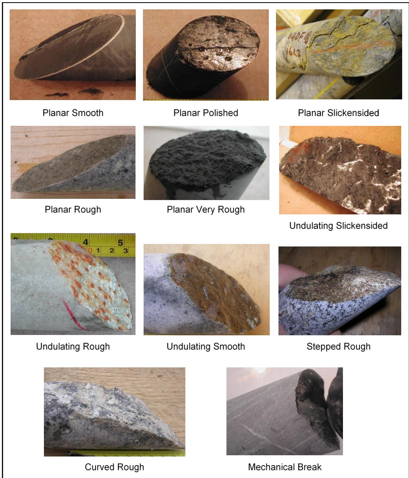
Figure A8: Examples of Discontinuity Shape and Roughness
