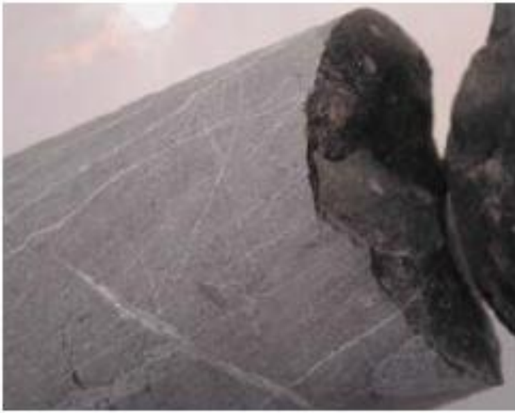
Figure A1: Example of Mechanical Break
