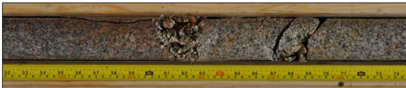
Figure 7 : Slightly weathered horizon at approximately 41.5 m depth observed in IG_BH01
