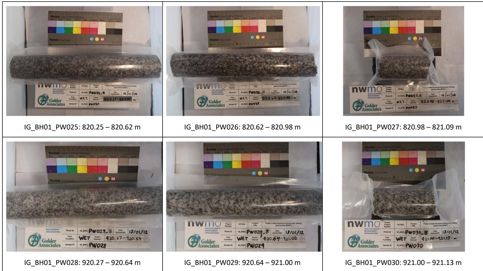
**Figure A-2: Laboratory documentation of core samples for porewater characterization sent to Hydroisotop; photos were taken right after unpacking**
