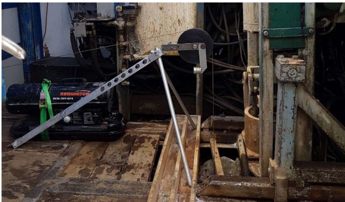
Figure 5: Borehole wireline tripod and wheel
