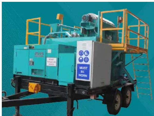
Figure 7: Typical Solids Recovery Unit (Courtesy AMC)
