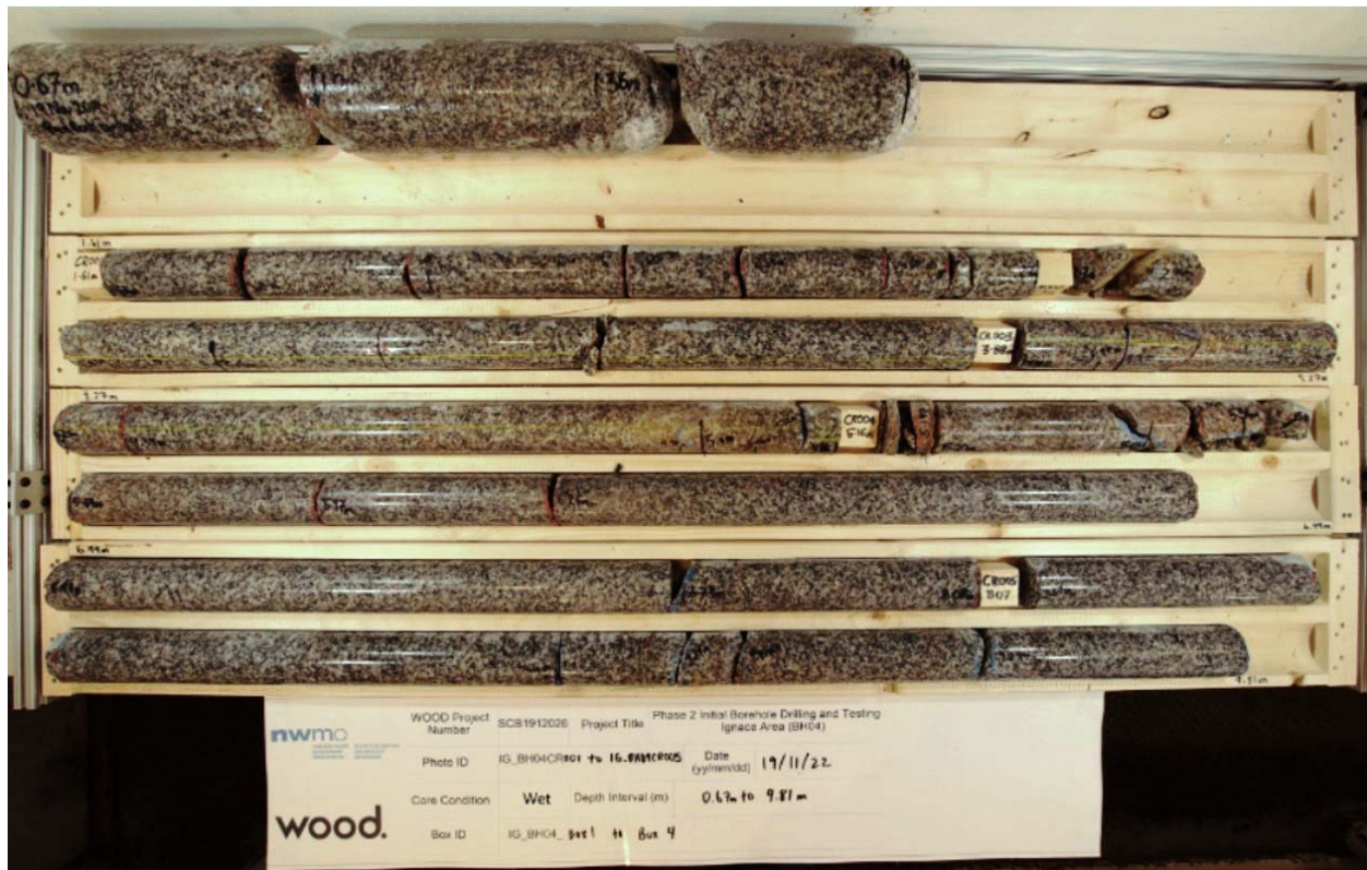
Figure 10: IG_BH04 : First core boxes illustrating PQ core and broken HQ3 core zone cased (5.45 and 5.69 m)
