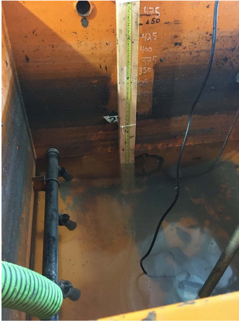
Figure 26: Measuring Tape Installed in STS Tank
