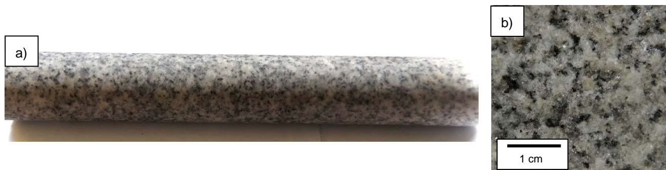
Figure 10: Sample IG_BH03_PW014 (669.2 mbgs (down hole)): a) Macroscopic appearance of the core, b) Macroscopic appearance of the core section PW0014 used for thin section production c) Overview of the mineral assemblage under transmitted, cross-polarized light, d) Overview of the mineral assemblage under transmitted plane-polarized light, e) Unaltered quartz and weakly to moderately altered plagioclase under transmitted, cross-polarized light, f) Sericitized plagioclase, weakly altered biotite partially replaced by epidote/clinozoisite and unaltered alkali feldspar under transmitted, cross-polarized light, g) Weakly altered biotite, and highly altered plagioclase on unaltered alkali feldspar under transmitted, cross-polarized light, h) Unaltered biotite with undefined grain boundaries on unaltered alkali feldspar showing microcline twinning under transmitted, cross-polarized light, i) Weakly to moderately altered plagioclase with strong zonation and unaltered alkali feldspar under transmitted, cross-polarized light, k) Sericitized plagioclase and unaltered alkali feldspar with microcline twinning under transmitted, cross-polarized light.
