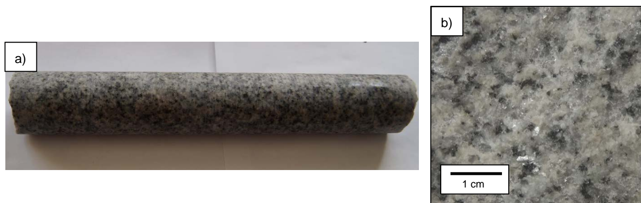
Figure 4: Sample IG_BH03_PW002 (242.0 mbgs (down hole)): a) Macroscopic appearance of the core, b) Macroscopic appearance of the core section PW002 used for thin section production c) Overview of the mineral assemblage under transmitted, cross-polarized light, d) Overview of the mineral assemblage under transmitted plane-polarized light, e) Chloritized biotite in association with weakly altered plagioclase containing bladed muscovite and granular epidote/clinozoisite under transmitted, cross-polarized light, f) Plagioclase with core containing epidote/clinozoisite under transmitted, cross-polarized light, g) Sericitized plagioclase imbedded in unaltered alkali feldspar under transmitted, cross-polarized light, h) Biotite partially replaced by epidote/clinozoisite and sericitized plagioclase under transmitted, cross-polarized light, i) Zoned plagioclase sericitized in the core and free of alteration products at the rim under transmitted, cross-polarized light, k) Altered plagioclase and unaltered quartz and alkali feldspar under transmitted, cross-polarized light.
