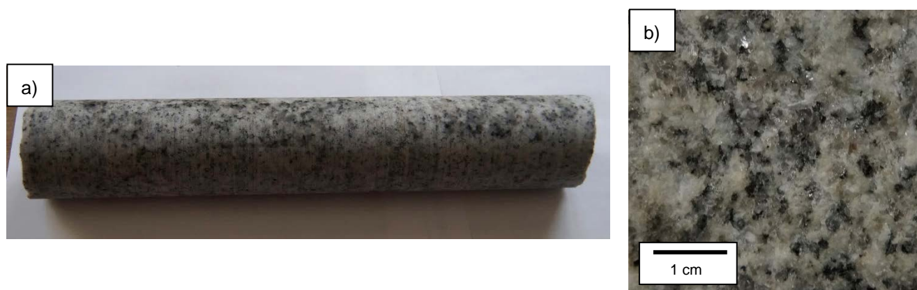
Figure 5: Sample IG_BH03_PW003 (345.2 mbgs (down hole)): a) Macroscopic appearance of the core, b) Macroscopic appearance of the core section PW003 used for thin section production c) Overview of the mineral assemblage under transmitted, cross-polarized light, d) Overview of the mineral assemblage under transmitted plane-polarized light, e) Sericitized plagioclase, weakly altered biotite and unaltered quartz under transmitted, cross-polarized light, f) Highly altered plagioclase imbedded in unaltered alkali feldspar under transmitted, cross-polarized light, g) Quartz cluster without alteration products and sericitization of sericitized core of plagioclase crystal under transmitted, cross-polarized light, h) Weakly chloritized biotite partially replaced by epidote/clinozoisite, sericitized plagioclase and unaltered quartz under transmitted, cross-polarized light, i) Altered biotite partially replaced by epidote/clinozoisite under transmitted, cross-polarized light, k) Needle like fine grained sericite and granular fine grained epidote/clinozoisite in microfissures of plagioclase under transmitted, cross-polarized light.
