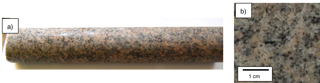
Figure 11: Sample IG_BH03_PW015 (771.6 mbgs (down hole)): a) Macroscopic appearance of the core, b) Macroscopic appearance of the core section PW0015 used for thin section production c) Overview of the mineral assemblage under transmitted, cross-polarized light, d) Overview of the mineral assemblage under transmitted plane-polarized light, e) Highly altered plagioclase in association with biotite and epidote/clinozoisite under transmitted, cross-polarized light, f) Moderately altered plagioclase with mainly granular epidote/clinozoisite in the core, unaltered biotite and epidote/clinozoisite under transmitted, cross-polarized light, g) Unaltered quartz and alkali feldspar with microcline twining and altered plagioclase under transmitted, cross-polarized light, h) Altered plagioclase in association with weakly altered biotite and epidote/clinozoisite under transmitted, cross-polarized light, i) Unaltered biotite and quartz with open grain boundaries under transmitted, cross-polarized light, k) Chloritized biotite partially replaced by epidote/clinozoisite under transmitted, cross-polarized light.
