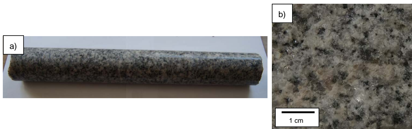
Figure 6: Sample IG_BH03_PW005 (459.2 mbgs (down hole)): a) Macroscopic appearance of the core, b) Macroscopic appearance of the core section PW005 used for thin section production c) Overview of the mineral assemblage under transmitted, cross-polarized light, d) Overview of the mineral assemblage under transmitted plane-polarized light, e) Sericitized plagioclase, chloritized biotite and unaltered alkali feldspar under transmitted, cross-polarized light, f) Quartz cluster with open grain boundaries under transmitted, cross-polarized light, g) Moderately altered plagioclase with alteration products mainly in the core and unaltered alkali feldspar under transmitted, cross-polarized light, h) Chloritized biotite with margin of fine grained epidote/clinozoisite on unaltered alkali feldspar under transmitted, cross-polarized light, i) Altered plagioclase with fine grained epidote/clinozoisite inclusions under transmitted, cross-polarized light, k) Needle like fine grained sericite and bladed muscovite inclusions in altered plagioclase under transmitted, cross-polarized light.
