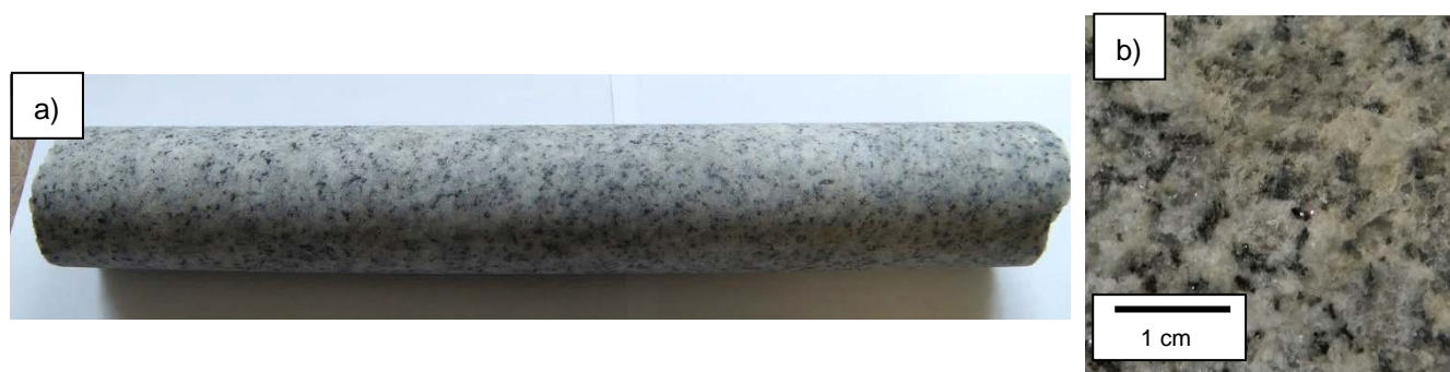
Figure 12: Sample IG_BH03_PW017 (880.4 mbgs (down hole)): a) Macroscopic appearance of the core, b) Macroscopic appearance of the core section PW0017 used for thin section production c) Overview of the mineral assemblage under transmitted, cross-polarized light, d) Overview of the mineral assemblage under transmitted plane-polarized light, e) Altered plagioclase and biotite on unaltered alkali feldspar showing microcline twinning under transmitted, cross-polarized light, f) Weakly altered plagioclase with granular epidote/clinozoisite in the core of the crystal and unaltered alkali feldspar under transmitted, cross-polarized light, g) Weakly altered plagioclase with bladed muscovite inclusions and lamellar twinning under transmitted, cross-polarized light, h) Highly sericitized plagioclase and weakly altered biotite partially replaced by epidote/clinozoisite under transmitted, cross-polarized light, i) Microfissures of plagioclase filled with needle like very fine grained sericite and granular epidote/clinozoisite under transmitted, cross-polarized light, k) Weakly altered biotite with margin of muscovite at sutural grain boundary and epidote/clinozoisite under transmitted, cross-polarized light.
