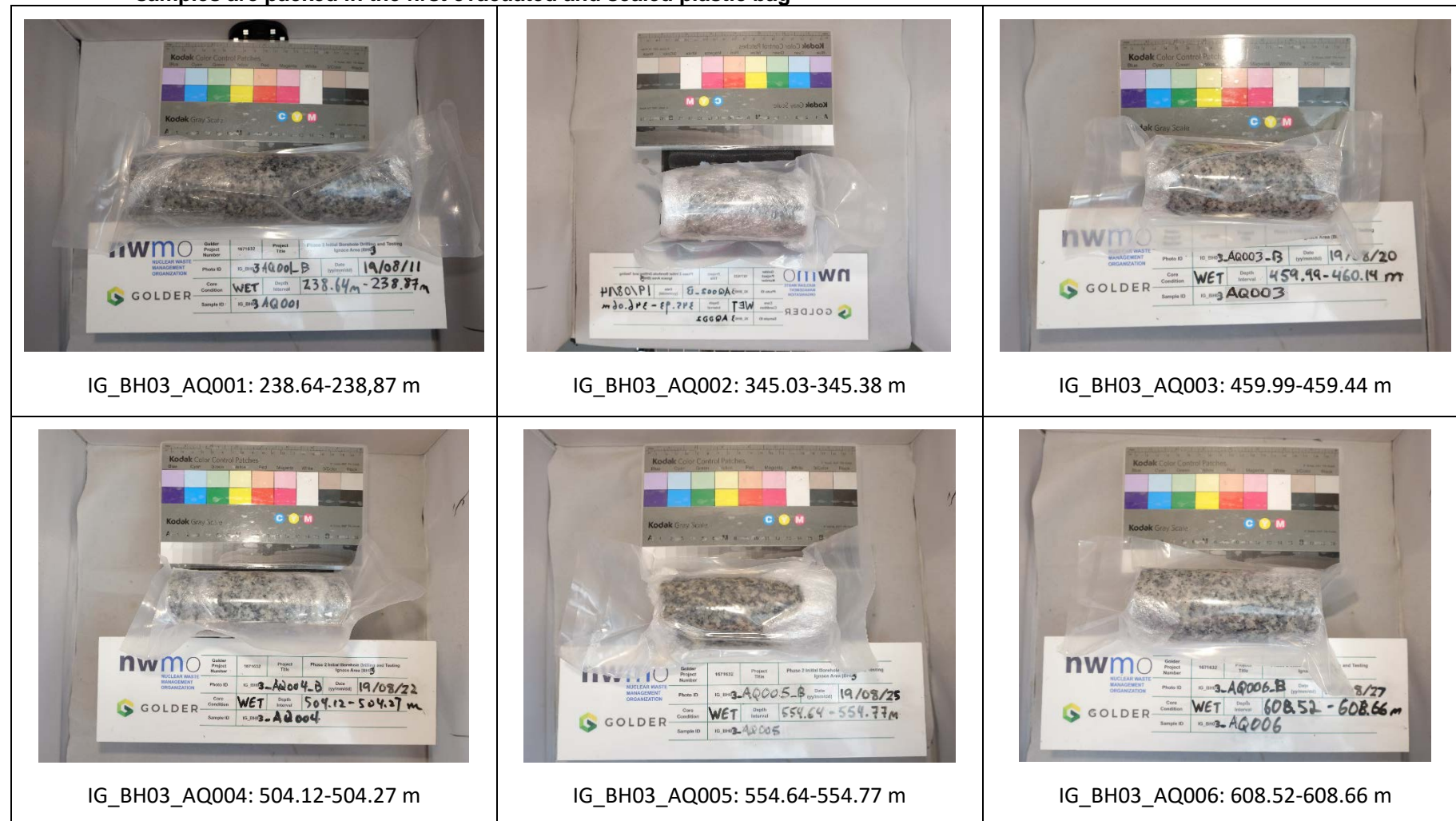
Figure A-1: On site documentation of core samples for porewater characterization sent to Hydroisotop (photos provided by Golder); Core samples are packed in the first evacuated and sealed plastic bag
