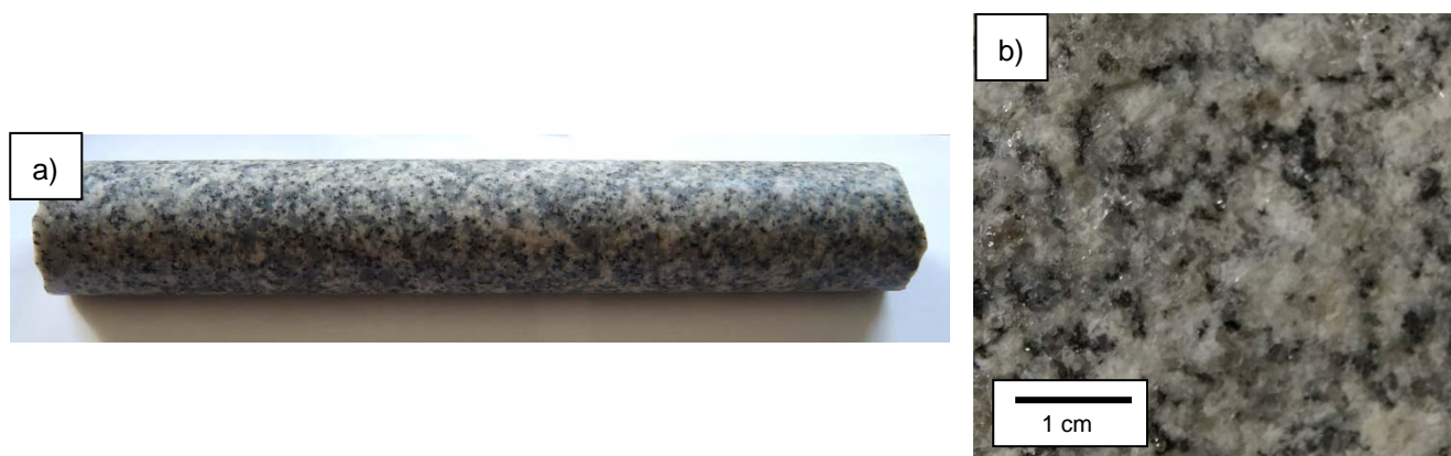
Figure 7: Sample IG_BH03_PW007 (503.9 mbgs (down hole)): a) Macroscopic appearance of the core, b) Macroscopic appearance of the core section PW007 used for thin section production c) Overview of the mineral assemblage under transmitted, cross-polarized light, d) Overview of the mineral assemblage under transmitted plane-polarized light, e) Sericitized plagioclase, weakly altered biotite with margin of fine grained muscovite and unaltered alkali feldspar under transmitted, cross-polarized light, f) Sericitized plagioclase and biotite under transmitted, cross-polarized light, g) Sericitized plagioclase in association with weakly altered biotite and epidote/clinozoisite under transmitted, cross-polarized light, h) Quartz cluster with open grain boundaries under transmitted, cross-polarized light, i) Chloritized biotite partially replaced by epidote/clinozoisite under transmitted, cross-polarized light, k) Plagioclase containing fine grained epidote/clinozoisite under transmitted, cross-polarized light
