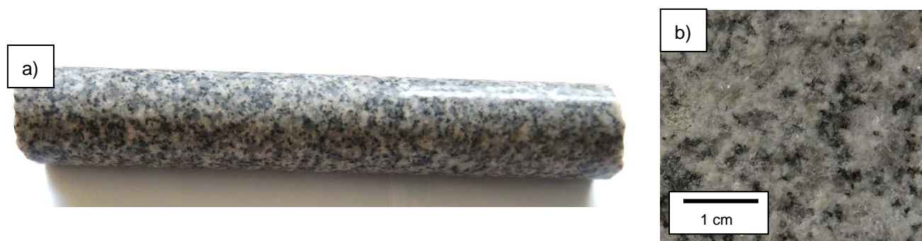
Figure 9: Sample IG_BH03_PW011 (608.8 mbgs (down hole)): a) Macroscopic appearance of the core, b) Macroscopic appearance of the core section PW011 used for thin section production c) Overview of the mineral assemblage under transmitted, cross-polarized light, d) Overview of the mineral assemblage under transmitted plane-polarized light, e) Quartz cluster with open grain boundaries and unaltered biotite under transmitted, cross-polarized light, f) Weakly altered plagioclase and unaltered quartz under transmitted, cross-polarized light, g) Unaltered quartz and moderately altered plagioclase containing granular epidote/clinozoisite under transmitted, cross-polarized light, h) Moderately altered plagioclase in association with weakly altered biotite and epidote/clinozoisite under transmitted, cross-polarized light, i) Weakly altered plagioclase, weakly chloritized biotite and epidote/clinozoisite under transmitted, cross-polarized light, k) Weakly altered biotite and margin of muscovite at sutural grain boundaries under transmitted, cross-polarized light.
