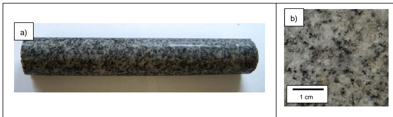
Figure 13: Sample IG_BH03_PW019 (984.7 mbgs (down hole)): a) Macroscopic appearance of the core, b) Macroscopic appearance of the core section PW0019 used for thin section production c) Overview of the mineral assemblage under transmitted, cross-polarized light, d) Overview of the mineral assemblage under transmitted plane-polarized light, e) Altered plagioclase and weakly altered biotite next to unaltered quartz and alkali feldspar showing microcline twinning under transmitted, cross-polarized light, f) Altered plagioclase and biotite in association with granular epidote/clinozoisite in the core of plagioclase and at plagioclase biotite grain boundaries under transmitted, cross-polarized light, g) Plagioclase with lamellar twinning containing alteration products mainly in the core next to weakly altered biotite, epidote/clinozoisite and unaltered quartz under transmitted, cross-polarized light, h) Plagioclase with varying degree of alteration under transmitted, cross-polarized light, i) Biotite in association with highly altered plagioclase partially replaced by epidote/clinozoisite and unaltered quartz under transmitted, cross-polarized light, k) Biotite partially replaced by epidote/clinozoisite and weakly altered plagioclase under transmitted, cross-polarized light.
