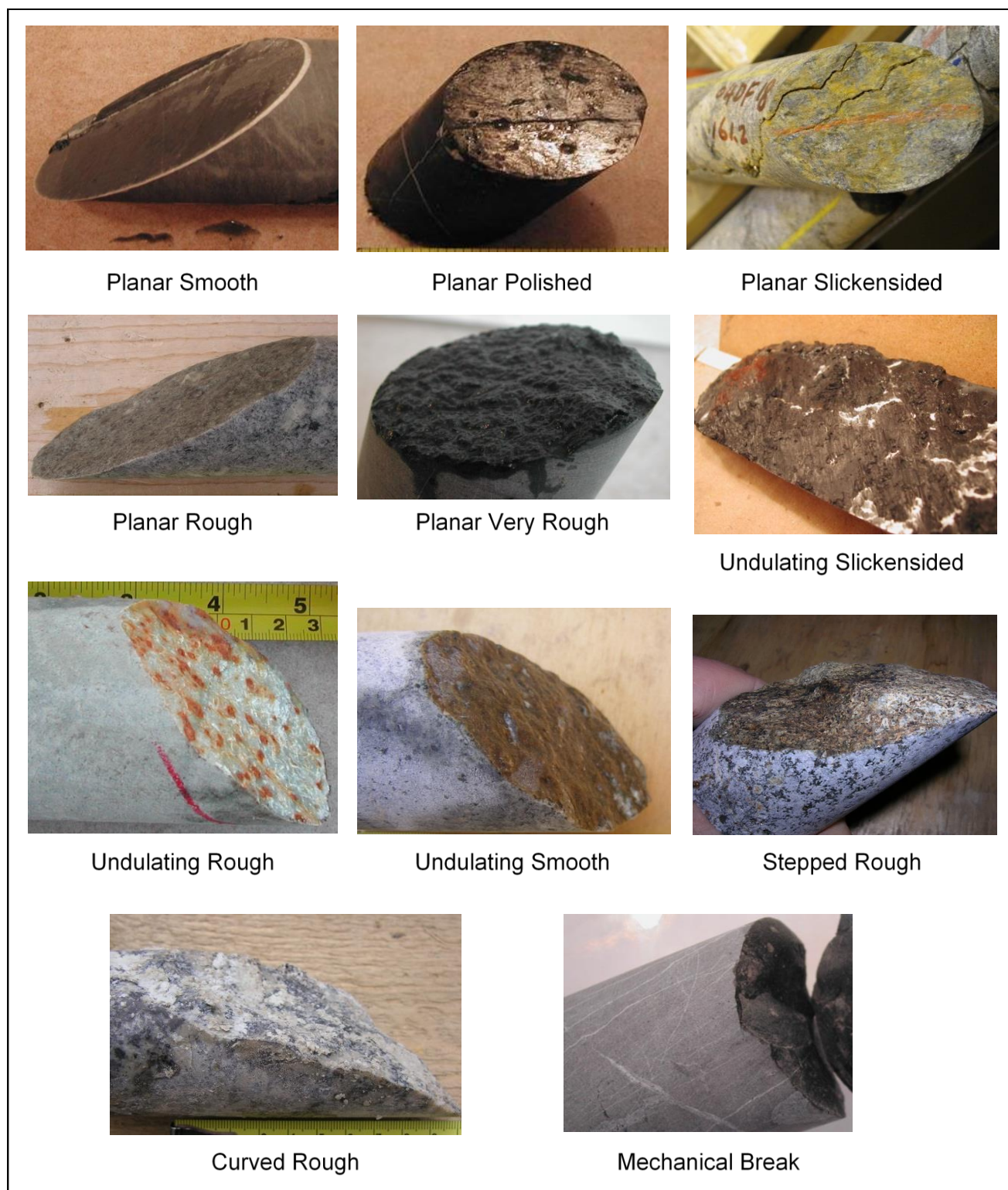
Figure 8: Examples of Discontinuity Shape and Roughness
