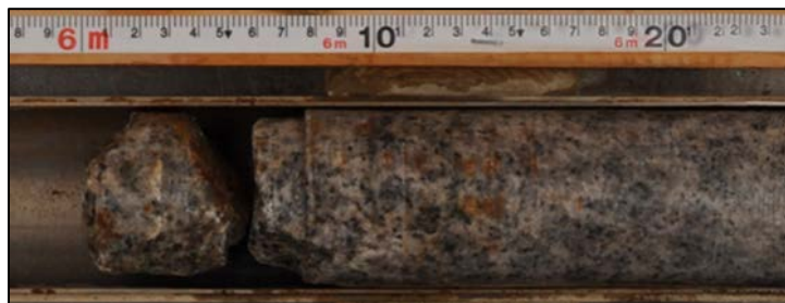
Figure 7 : Slightly weathered horizon at approximately 2.7 m depth observed in IG_BH02
