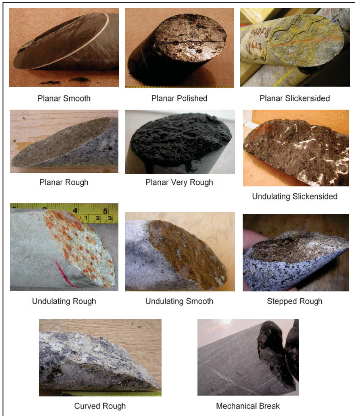
Figure 8: Examples of Discontinuity Shape and Roughness
