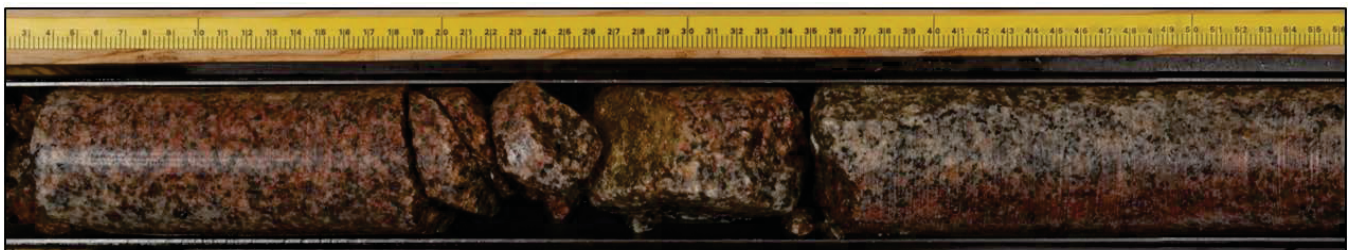
Figure 7 : Portion of 6.19 m wide zone of slightly weathered horizon at approximately 4.5 m depth along borehole observed in IG_BH03
