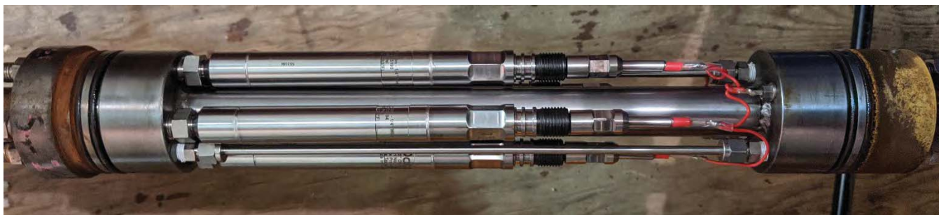
Figure 3: DataCan Gauge Carrier and Transducers with Outer Protective Casing Removed
