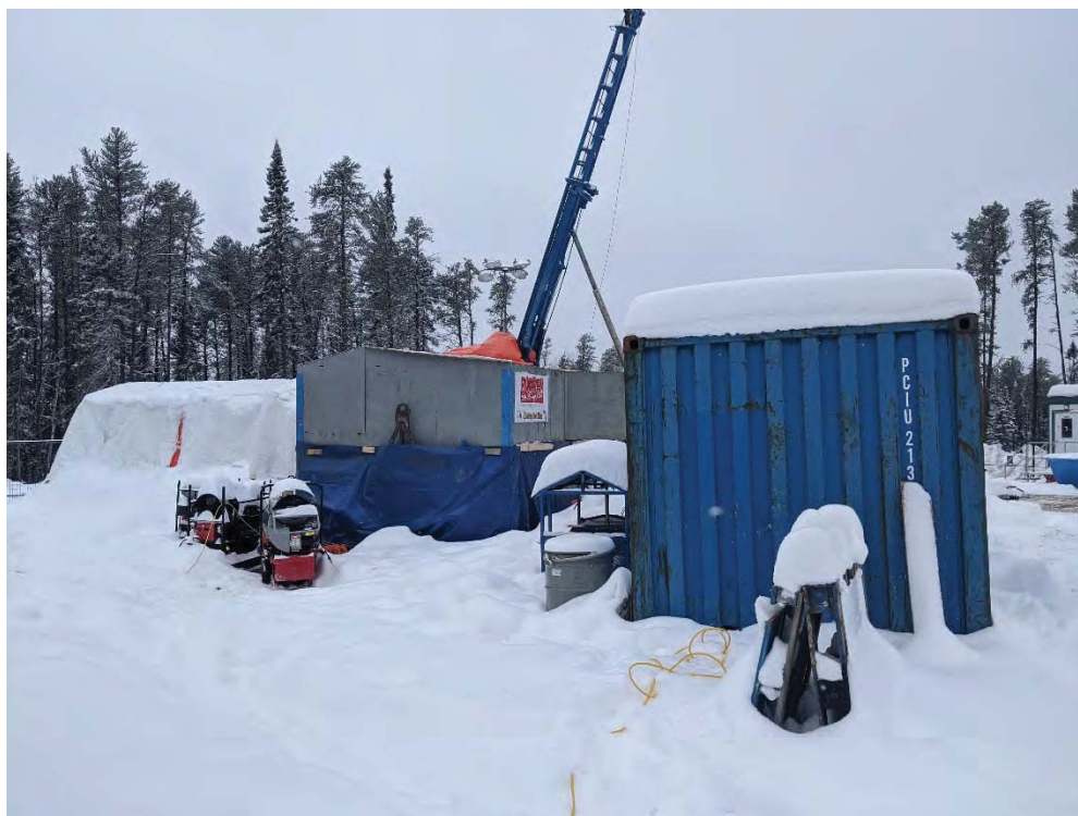
Photo 1 – Drill rig and insulated and heated tent (white) containing flat pack. Water tanks located in heated blue shipping container.
