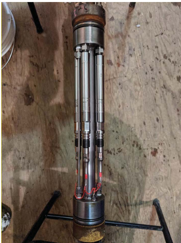
Photo 3 – DataCan pressure transducer tool carrier with outer protective casing removed.
