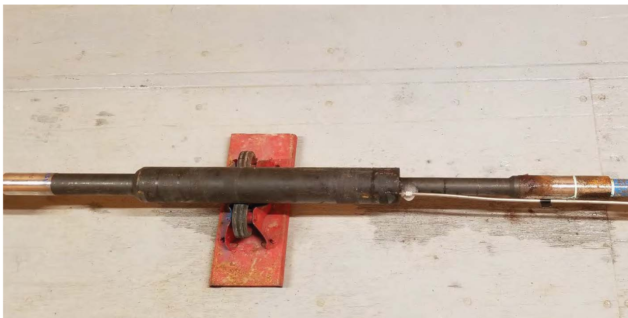
Photo 4 – Downhole shut-in valve (DHSIV) with stainless steel activation line ported in top of tool.
