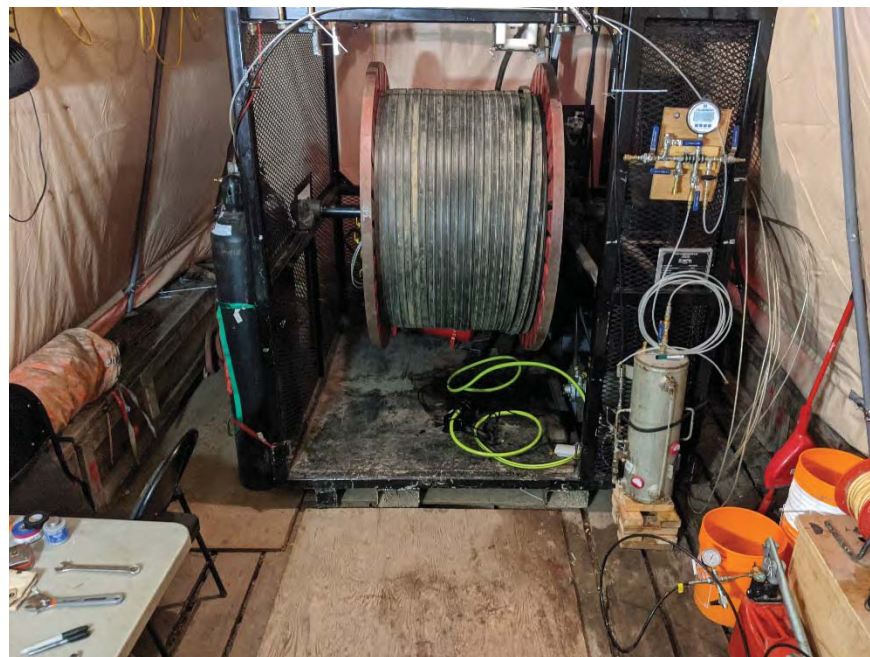
Photo 2 – Flat pack (center) with inflation manifold (upper right), inflation pressure vessel (lower right), nitrogen cylinders (center left), and DHSIV activation pump (lower right).
