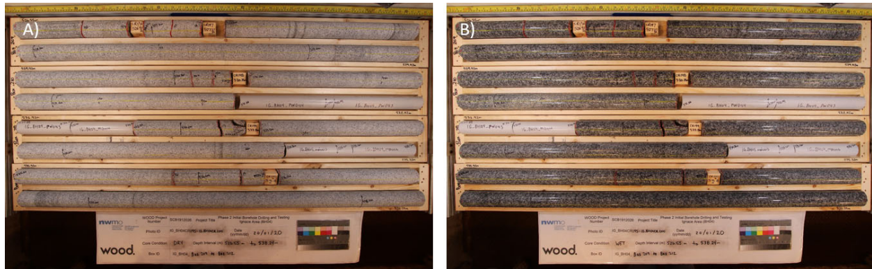
Figure 20: Boxed core photography of core boxes 209-212 (526.55-538.24 m). A) Dry and B) Wet
