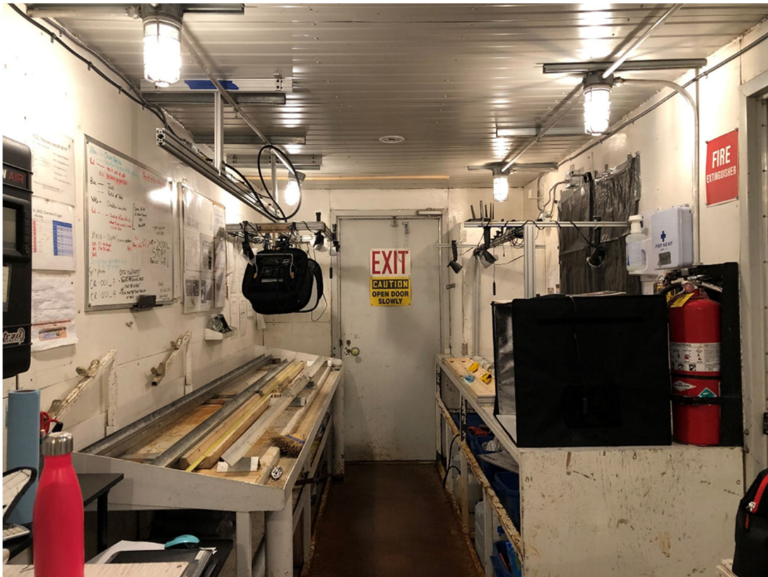
Figure 5: Core logging trailer, left side displays core split photography setup, far right side displays core box photograph set up and front right side shows sample and detailed structure photography setup (Light box)
