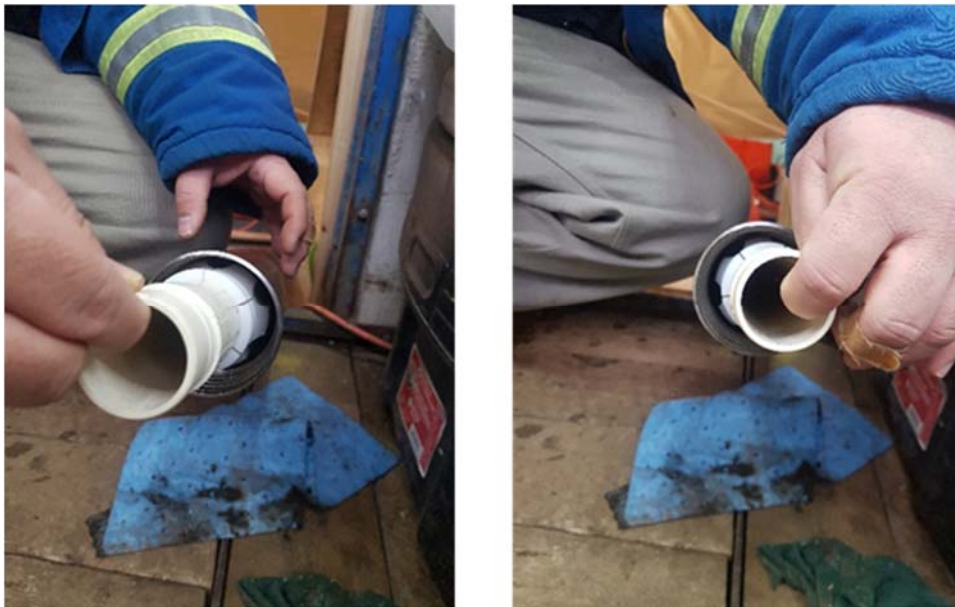
Figure 2: Illustration of how abrasion protector fits inside HQ rods
