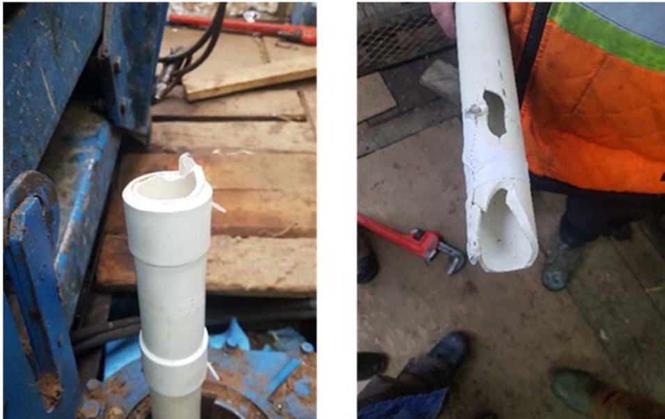
Figure 1: Broken Westbay PVC extension (top and bottom)
