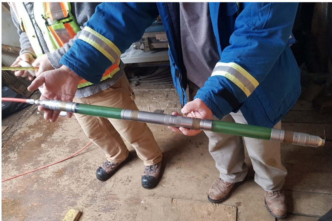
Figure 5: Photograph of joint testing and packer inflation tool
