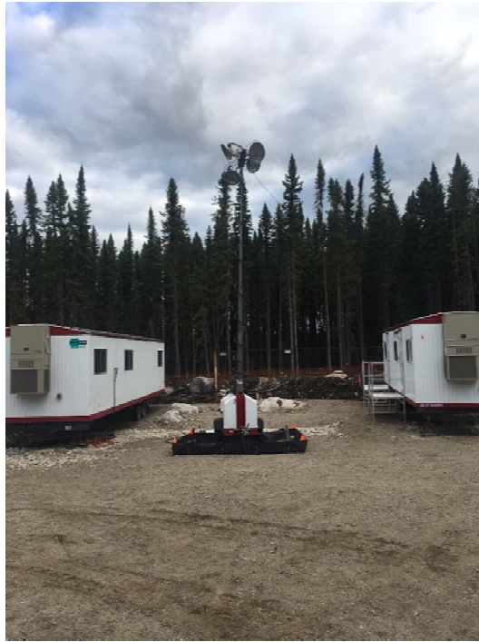
Photo 8: Facing north towards one of four 8-kilowatt light towers. Each light tower was placed in a secondary containment berm to capture any potential spills. The site cell phone signal booster is visible at the top of the light tower.
