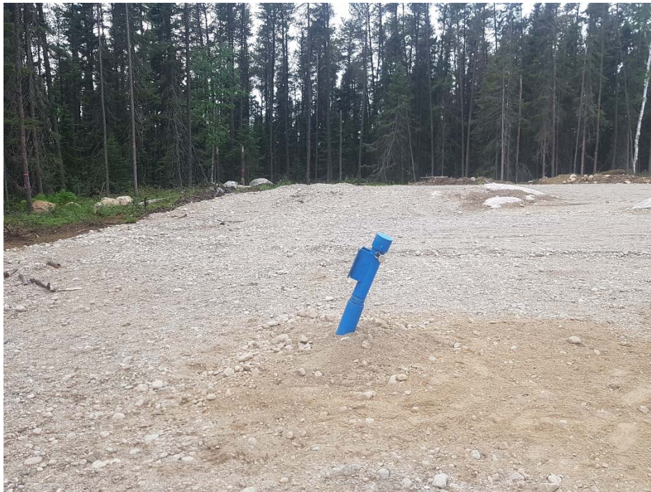
Photo 7: Facing east towards IG_BH03 with locking protective casing and monopod bracket, and backfilled drilling sump, July 7, 2020.
