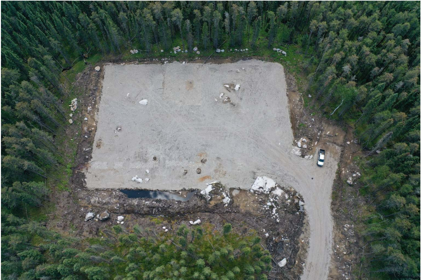
Photo 9: Aerial drone photo of the IG_BH03 site (facing south) following demobilization. Photo was taken in July 2020. Discolorations visible in the gravel fill were caused by recent digging to remove underground infrastructure.
