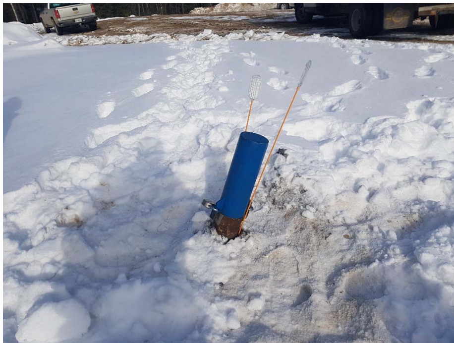
Photo 4: Facing northeast towards the lockable casing placed over the IG_BH02 drill collar on March 18, 2020.
