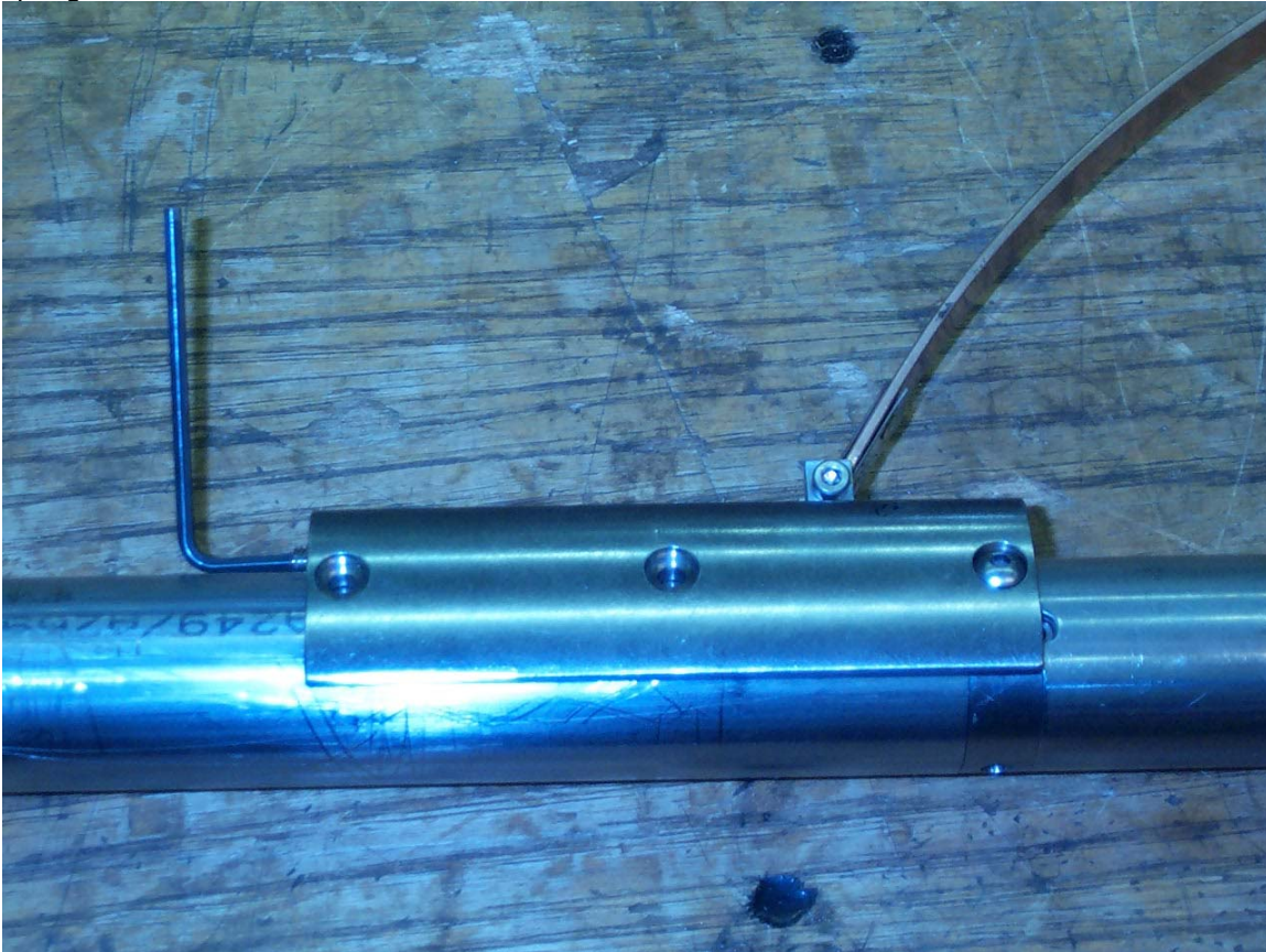
Figure 8 Top mount locating holes, and allen wrench used for tension spring changeout
