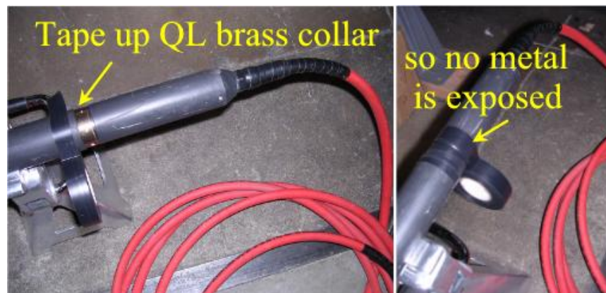
Figure 3-5 bridle connection and isolation
