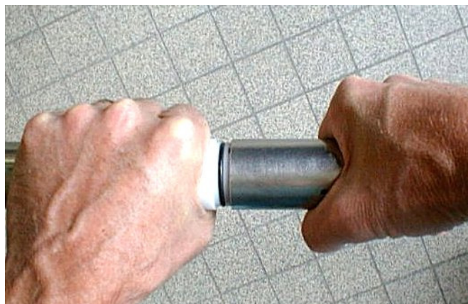
Figure 6-7 Unscrewing the bellows cover
