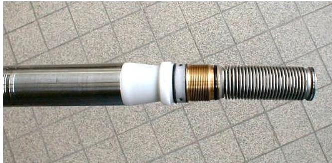
Figure 6-8 Bellows cover removed
