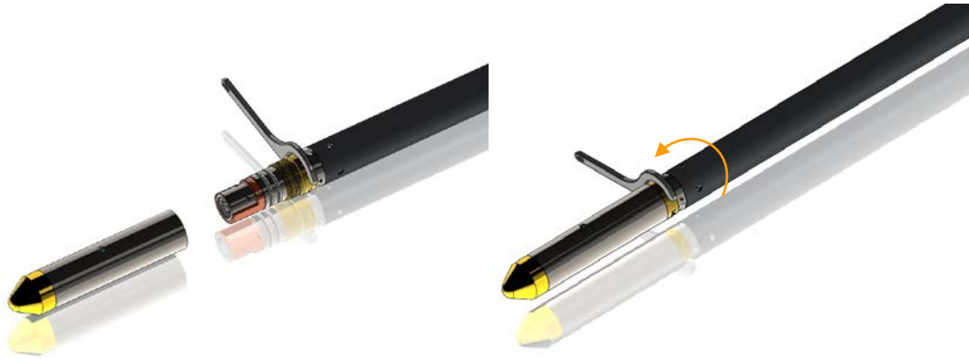
Figure 3-4 Attaching the QL40-Bottom Plug
