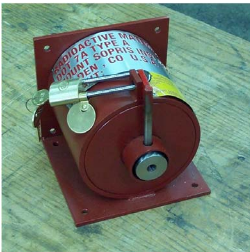
Shield with source and spacer installed
