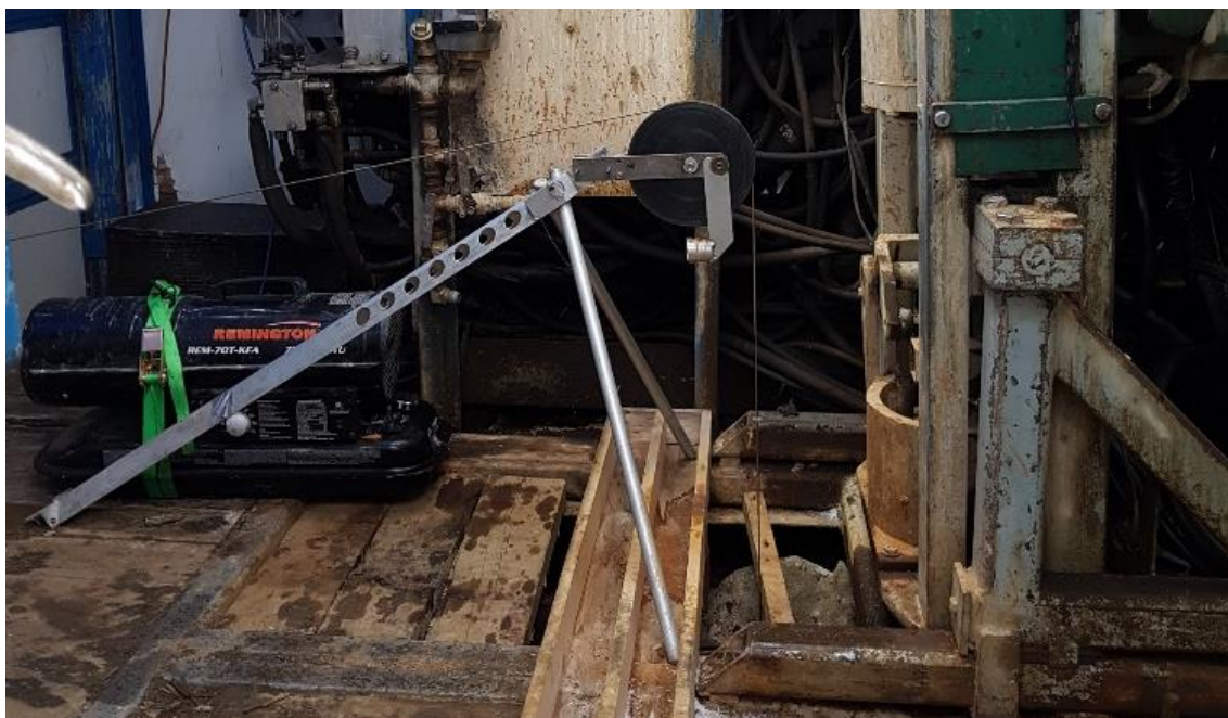
Figure 5: Borehole wireline tripod and wheel
