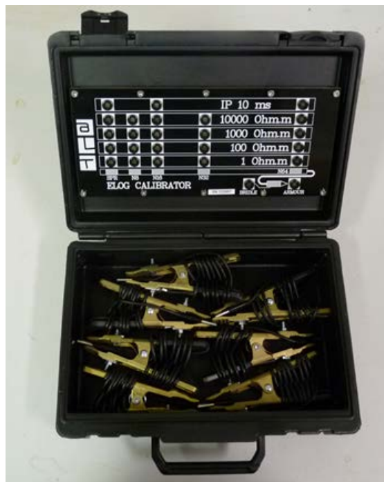
Figure 3-3 ELOG Calibrator, cables and clamps
