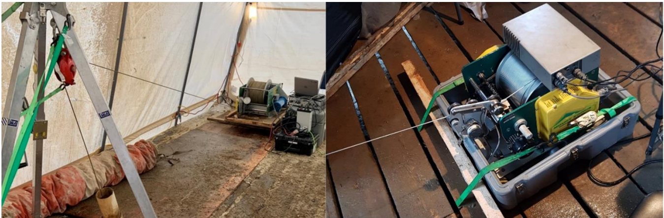
Figure 3: On the right: Mount Sopris 2MXA 1000m winch with Matrix logging box, on the left: Mount Sopris Instruments (MSI) 4WNA 1800m winch with WCA winch controller and SCOUT logging box.
