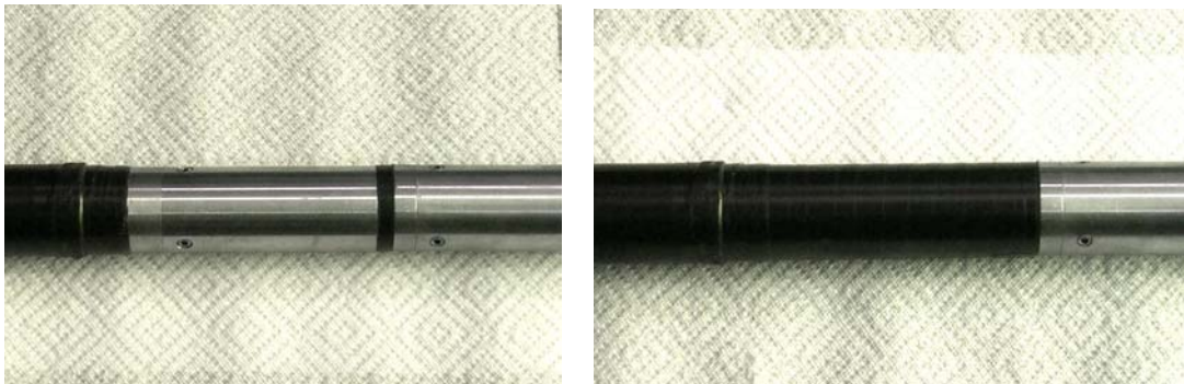
Figure 5: Proper isolation for resistivity measurement is shown in the view on the right.
