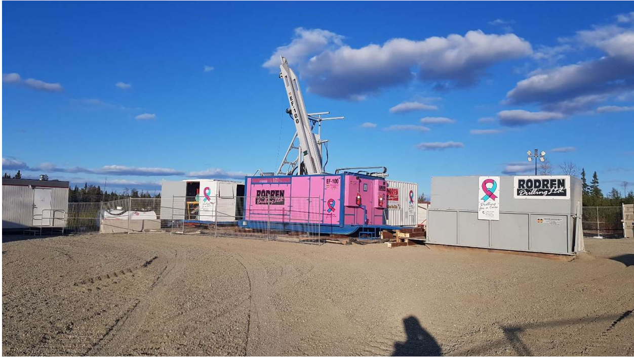
Photo 13 - Drill rig after positioning on IG_BH05 at the desired orientation.
