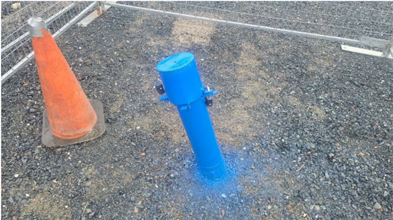
Photo 8 – IG_BH04 Surface casing spray painted blue with two locks provided by the NWMO - September 8, 2021.
