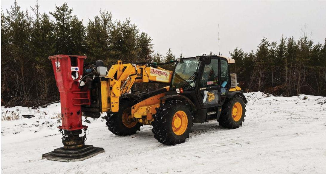
Figure 2. VIBSIST-3000 source being used on Line 4.
