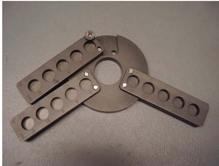
Figure 5-1 3 Arm Caliper, calibration Jig shown with one arm folded for ease of packaging
