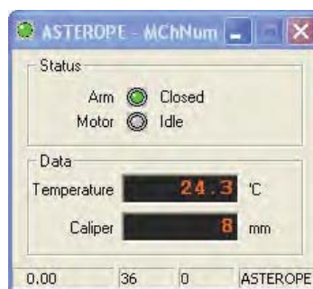
Figure 4-11 MChNum window display for arm fully closed
