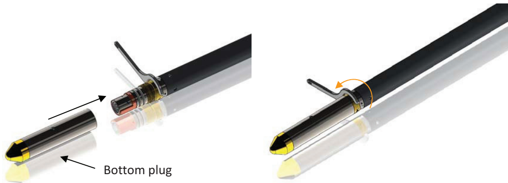
Figure 3-4 Attaching the QL40-Plug
