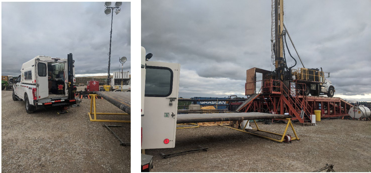
Figure 3 SB_BH02 Field Equipment Setup. Winchline extended from Colog truck over pulley on drill rig.
