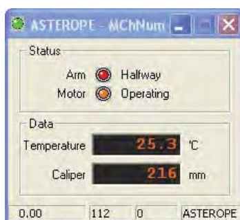
Figure 4-8 MChNum window to monitor the calliper opening process
