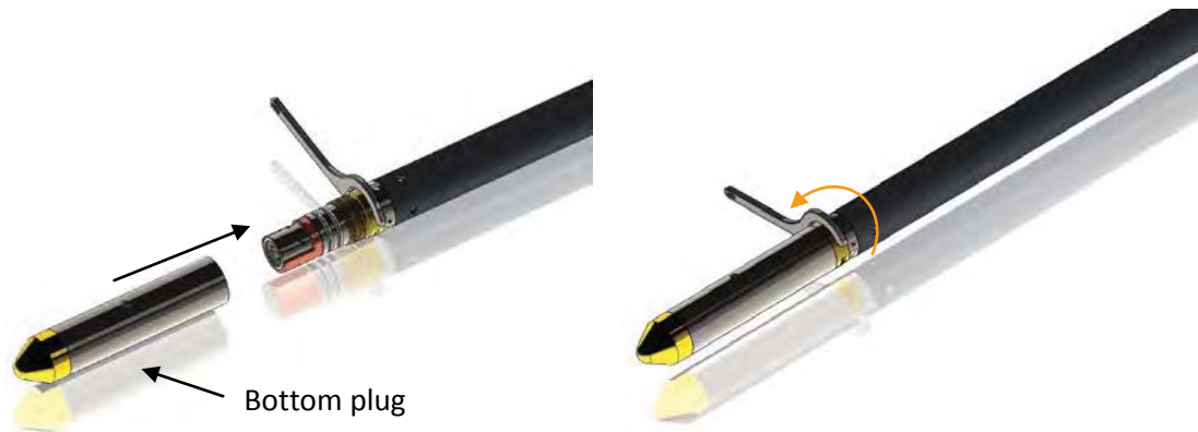
Figure 3-4 Attaching the QL40-Plug
