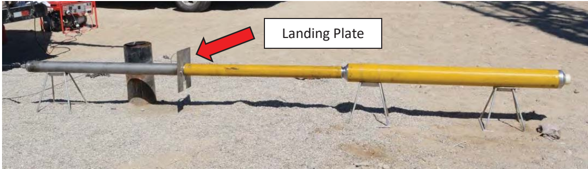
Figure 35: Landing plate (or C-plate) in position on a 3-section system.
