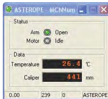
Figure 4-10 MChNum window indicates arms fully opened
