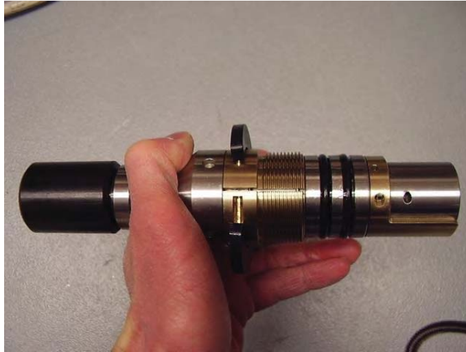
Figure 6-2 Disassembly of the locking ring –step 1
