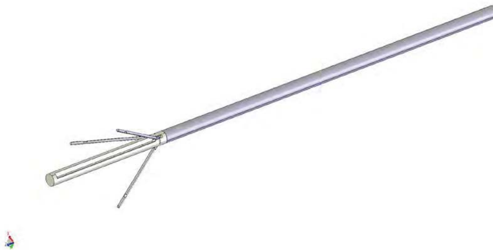
Figure 1-2 QL40 CAL 3-arm caliper probe
