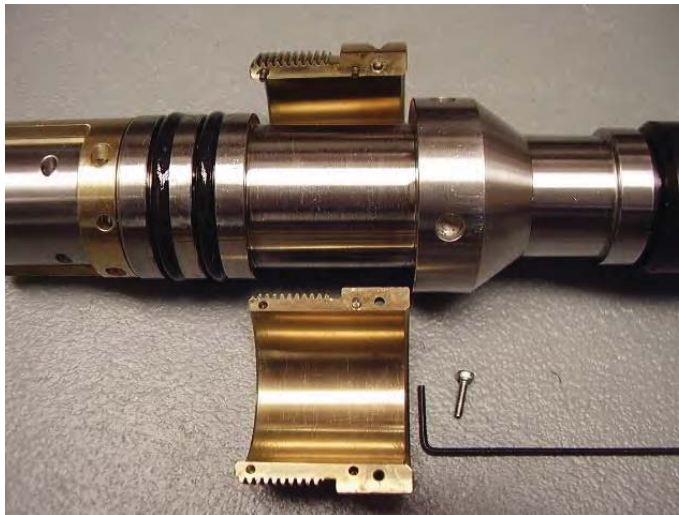
Figure 6-3 Disassembly of the locking ring –step 2
