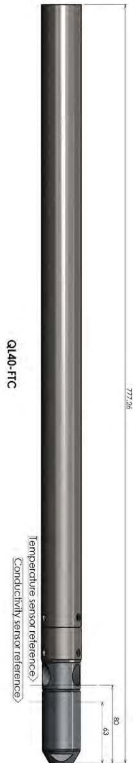
Figure 1-1 QL40 FTC Dimensions (bottom sub)
