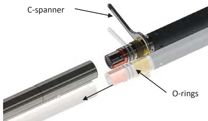
Figure 3-1 C-spanner and O-rings of QL connection
