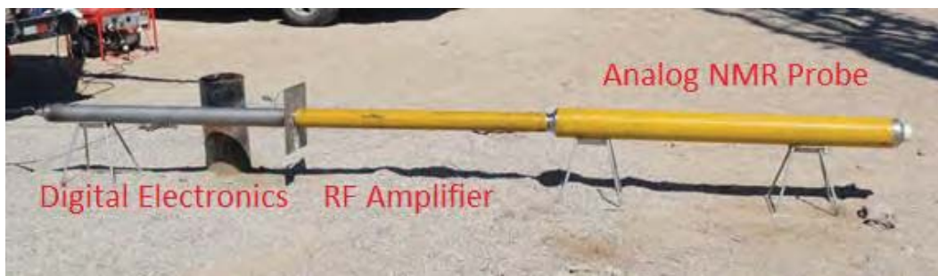
Figure 2: Example of Javelin Max downhole logging system (three-section), shown with 5.25-inch Analog MR Probe.
