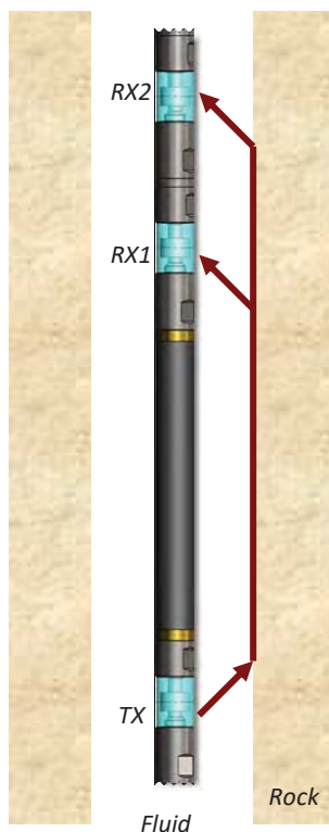
Figure 2-1 Typical wave path for a 1 transmitter and 2 receiver tool
