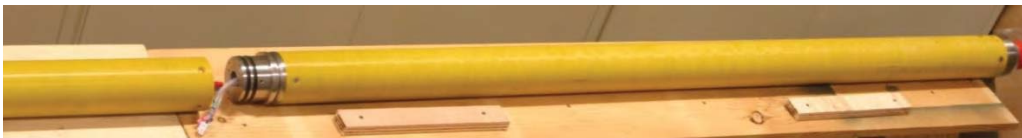
Figure 25: Connection between Power Module and Analog MR Probes.
