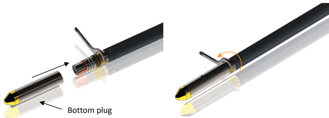
Figure 3-4 Attaching the QL40-Plug
