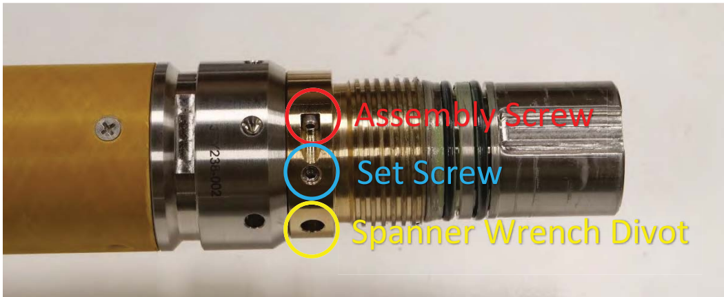
Figure 20: Three types of screws and holes on the threaded brass section of the Javelin Slim. (A) Spanner Wrench Divot – use to tighten and loosen the two sides of the Field Joint together. (B) Set Screws (2x) – tighten these to secure brass threaded section and prevent it from rotating. (C) Assembly Screws (2x) – do not remove these except to disassemble the brass threaded section (e.g., for cleaning or repair).
