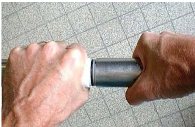
Figure 6-7 Unscrewing the bellows cover
