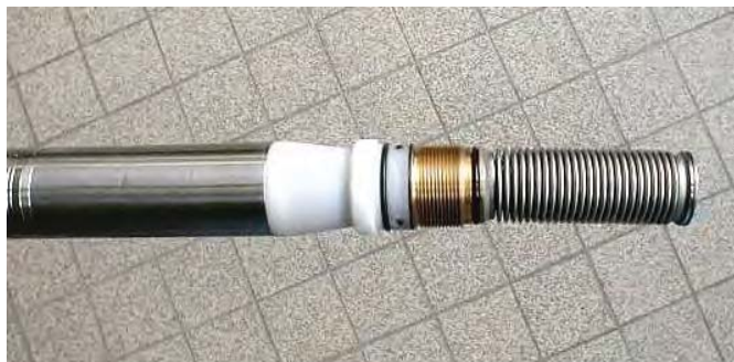
Figure 6-8 Bellows cover removed
