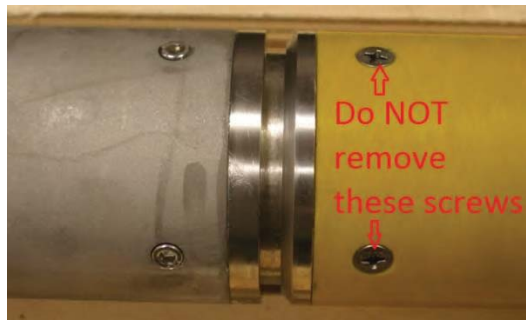
Figure 31: Completely assembled Double Joint between Digital Module and Power Module. Connect Socket Head Cap Screws (1/4-20 x 1/2") for securing Joint to Digital Module. Never remove the screws on the "downhole" side of the Double Joint.
