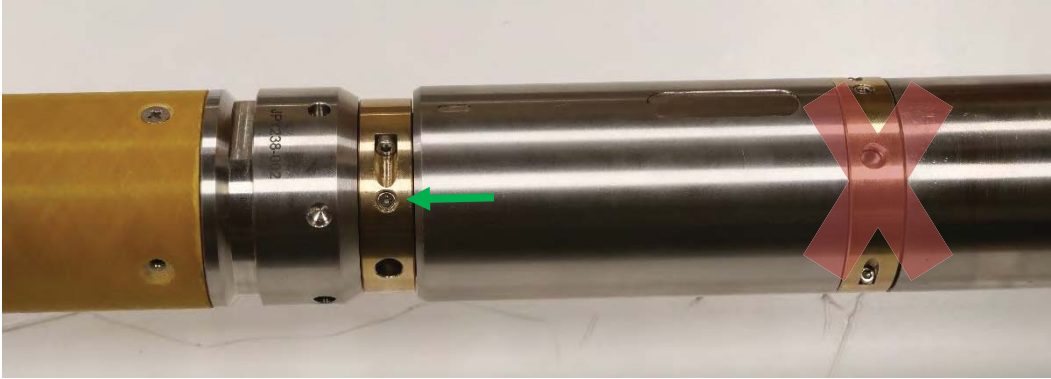
Figure 23: Field Joint connection of Javelin Slim completely made. Always tighten set screws prior to logging (green arrow; second set screw not pictured). Never adjust the upper (uphole) brass section.
