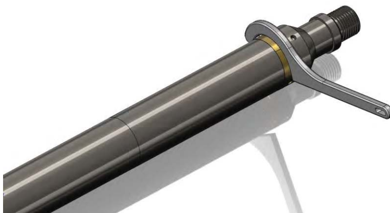
Figure 6-1 Removing the tool top
