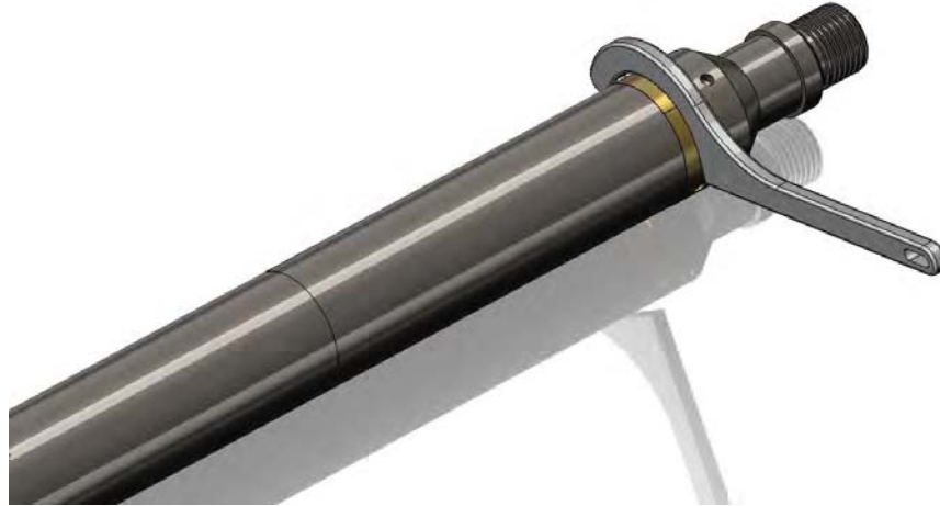
Figure 6-2 Removing the tool top
