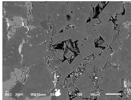
Inset A-1: Porosity likely created by volume change during dolomitization. Pores contain clay minerals. Bright white grains are pyrite, light grey is calcite and dark grey is dolomite.
