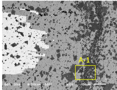
Location A: Calcite matrix (medium grey) has been overprinted by large grains of gypsum/anhydrite (light grey) and dolomite (dark grey). There is gypsum/anhydrite in the fracture near the top and minor pyrite (white) disseminated in the gypsum/anhydrite, in the calcite matrix and in the dolomite. Dolomitization is focused along the near vertical fracture at the right side.
