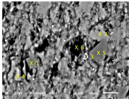
Inset A-1: Fine organic fragments (black) with clay minerals lining the pore walls. Numbers indicate locations of EDS analyses used to identify minerals 1) dolomite, 2) calcite, 3) sphene, 4) calcite, 5) dolomite, 6) organic fragment.
