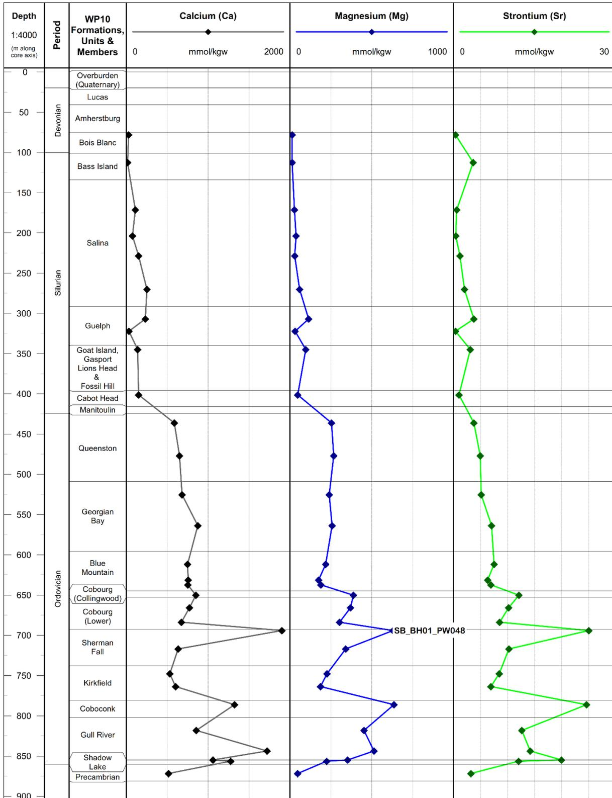
**Figure 4** Profile of Calcium, Magnesium, and Strontium Concentrations in Porewater from Vacuum Distillation, SB\_BH01 Core Samples. Sample SB\_BH01\_PW048 was noted to have exceptionally low water content and strong degassing of methane during sampling.
