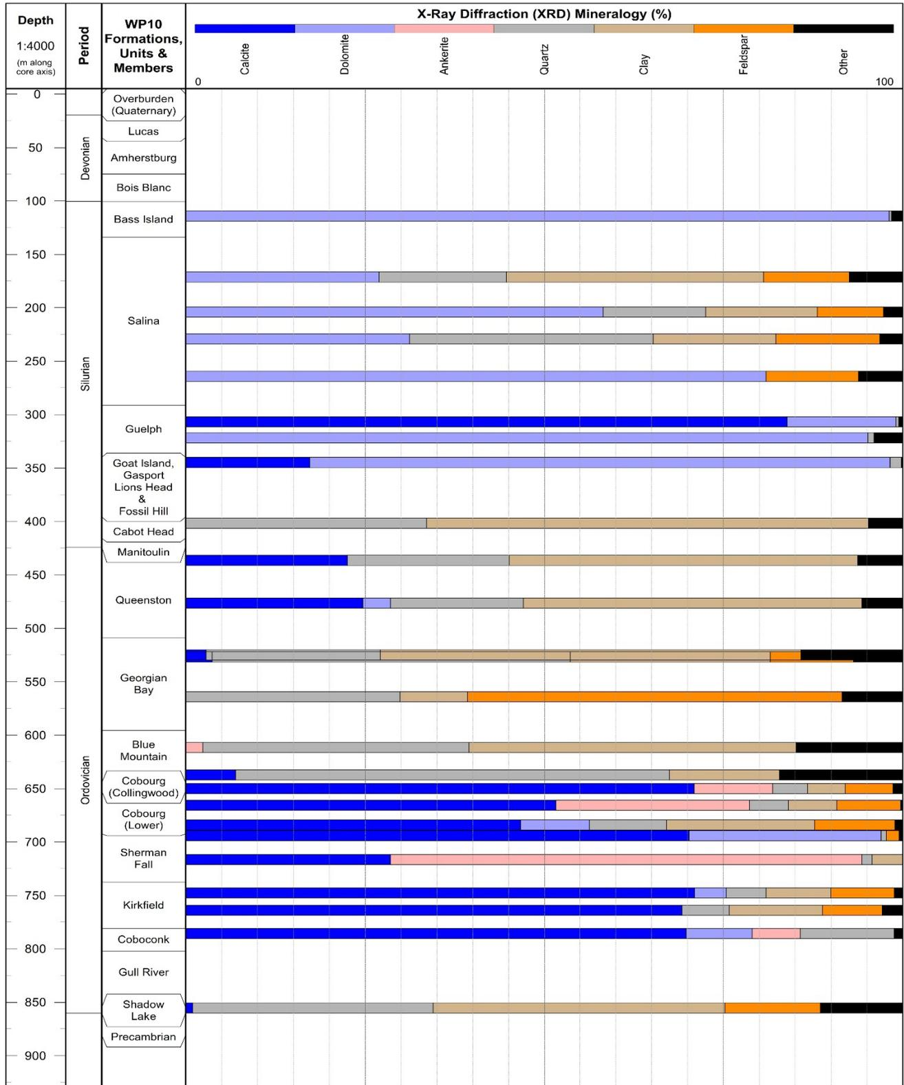
**Figure 11 Mineralogical Components, by X-Ray Diffraction, SB\_BH01 Core Samples**
