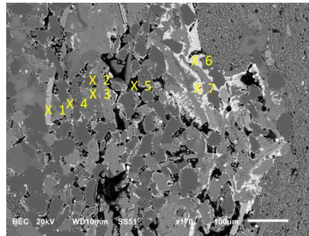
Inset A-1: Higher magnification images of the silty lens with organic fragments (black) and diagenetic pyrite. Numbers indicate locations of EDS analyses used to identify minerals 1) apatite (biogenic?), 2) quartz, 3) mixed Ca-Al-Mg-K silicates, 4) calcite, 5) organic fragment, 6) pyrite, 7) pyrite.
