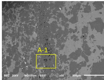
Location A: The boundary observed in the scanned image at left marks the change from relatively coarse calcite-rich matrix at the right to finer dolomite-rich matrix at left. Calcite is light grey, dolomite is dark grey. The dolomite-rich zone has higher porosity (inset) and contains greater abundance of pyrite (disseminated white grains).
