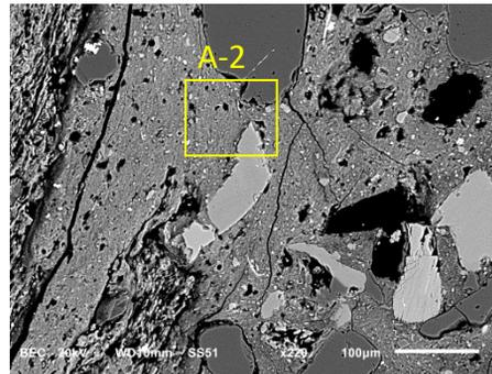
Inset A-1: Higher magnification image showing matrix with a mix detrital grains and cement with clay-composition (Mg-Fe-Si-Al-Ca-K). Clay minerals are evident in the higher magnification image (inset A-2) of the matrix at lower left.
