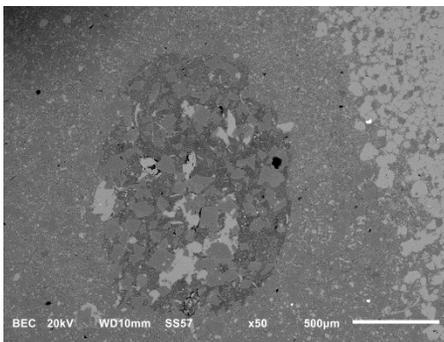
Location B: Siliceous, calcite-rich halo (medium grey) surrounding circular region with relatively large calcite and dolomite grains and organic material in largest pores.
