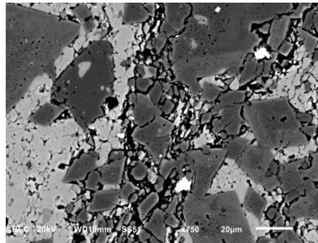
Inset A-1: Higher magnification image of the fracture. The micritic calcite matrix is light grey, pyrite grains are white and the dark grey crystals are dolomite. The fracture contains organics (black), and EDS analyses indicate that it is lined with clay minerals.
