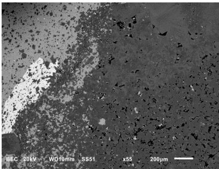
Location B: Calcite matrix and gypsum/anhydrite grain (upper left) are overprinted by dolomite to the point where the material on the right side of the image (oval-shaped features in the scanned colour image) is almost 100% dolomite with organic-filled pores.
