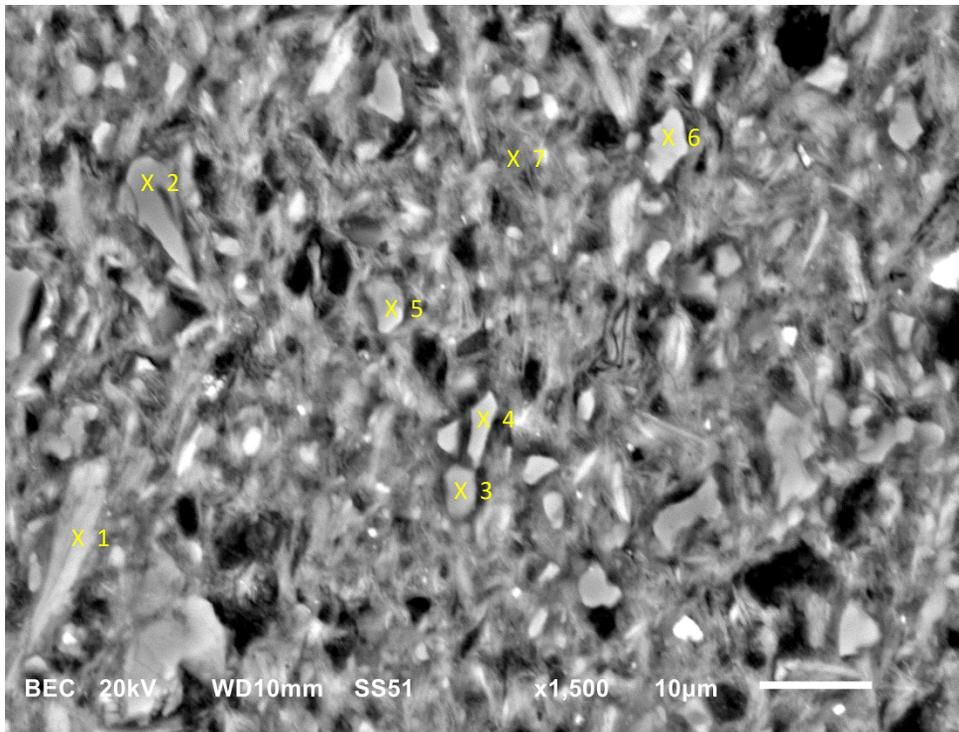
Location C: Very fine-grained shale with detrital minerals, mostly quartz, and clay minerals lining the pores. Numbers indicate locations of EDS analyses used to identify minerals 1) biotite, 2) quartz, 3) quartz, 4) quartz, 5) quartz, 6) K feldspar, 7) clay minerals.
