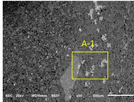
Location A: Boundary between relatively coarse- (left) and fine-grained (right) layers.
