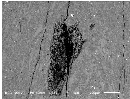
Location A: Organic material (black) infilling porous zone and cross-cutting fracture in micritic and bioclastic matrix.
