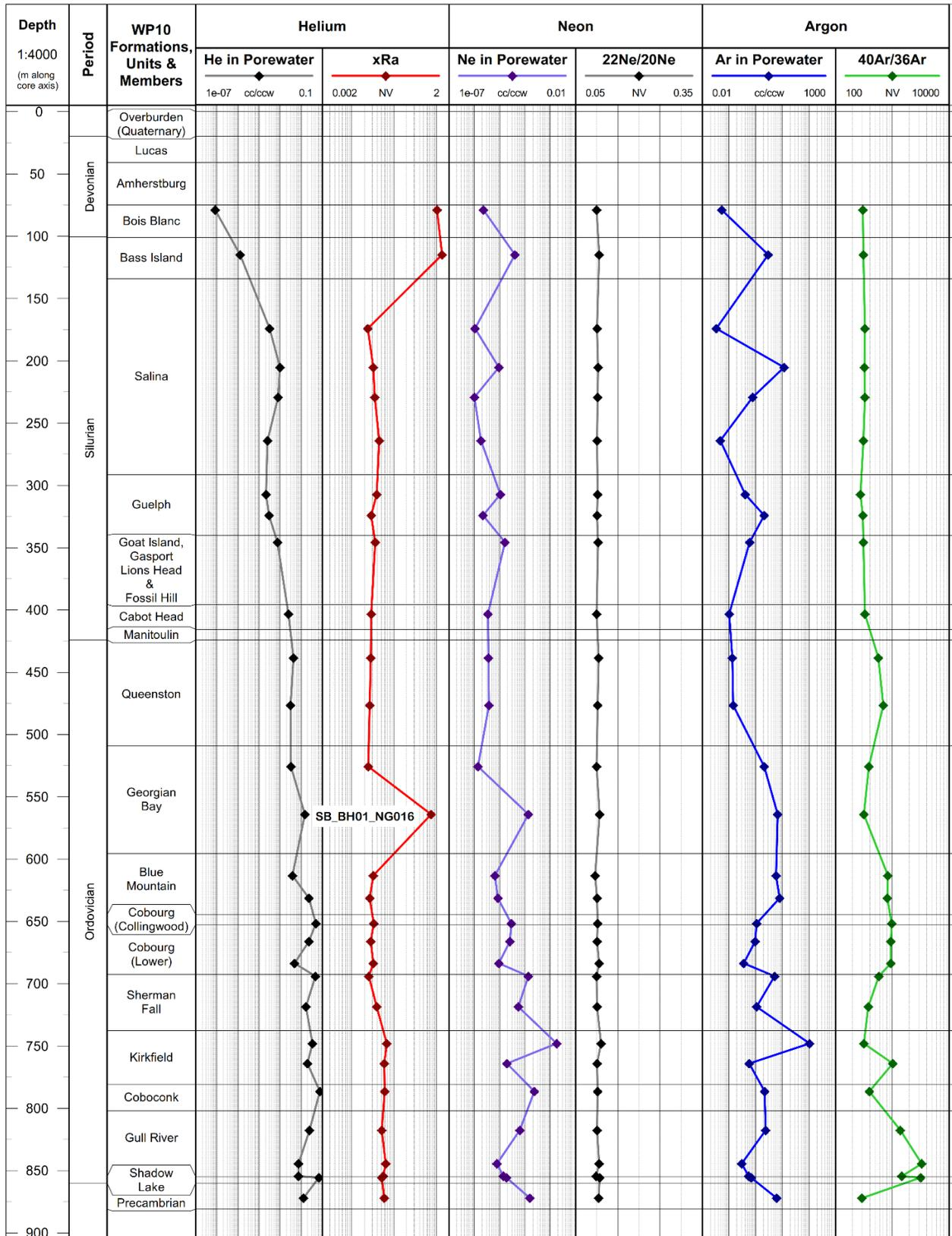
**Figure 9** Profile of Noble Gas (He, Ne, Ar) Concentrations and Isotopes for Porewater from SB\_BH01 Core Samples, xRa = Air-normalized  $^3\text{He}/^4\text{He}$  ratio.
