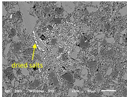
Location A: Light grey spots represent salts, mostly NaCl, precipitated from dried pore water.
