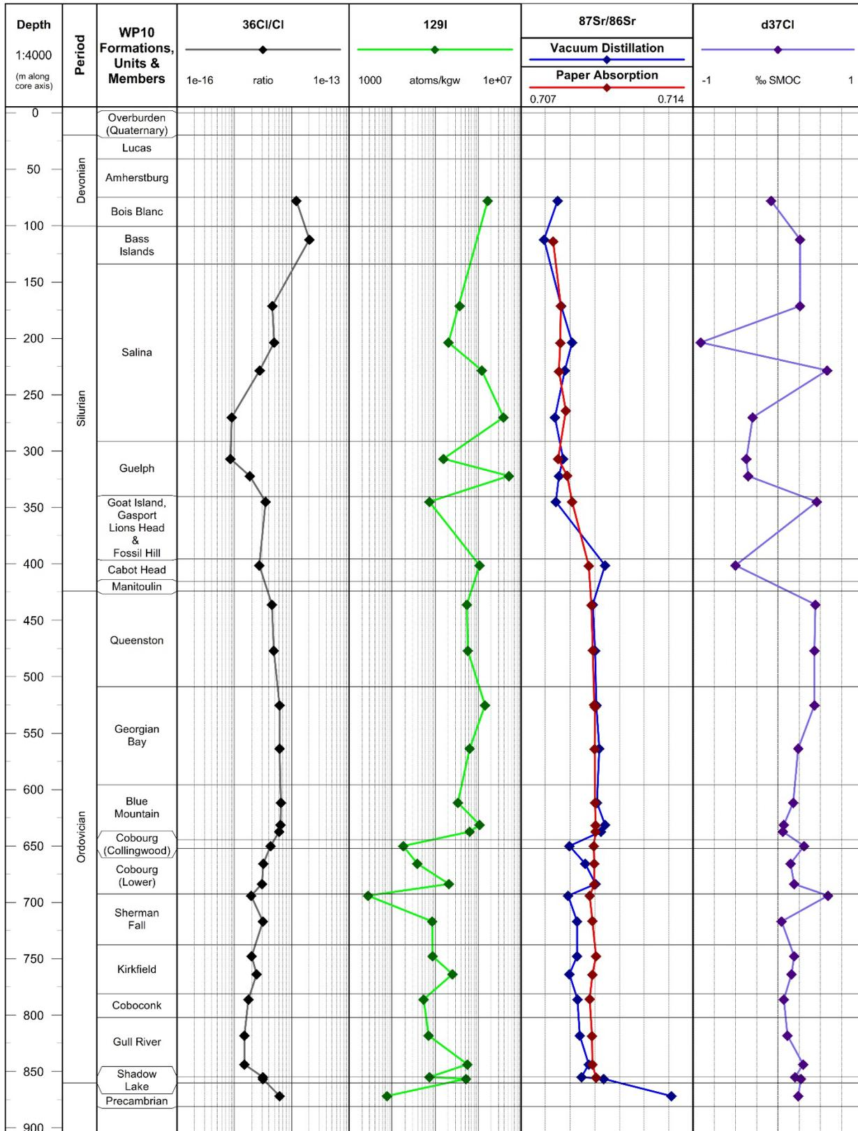
**Figure 8** Profile of  $^{36}\text{Cl}$ ,  $^{129}\text{I}$ ,  $^{87}\text{Sr}/^{86}\text{Sr}$ , and  $^{37}\text{Cl}$  Isotopic Results for Porewater from SB\_BH01 Core Samples
