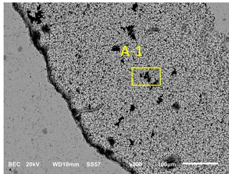
Location A: Porous microcrystalline calcite with organic material (black) infilling largest pores.
