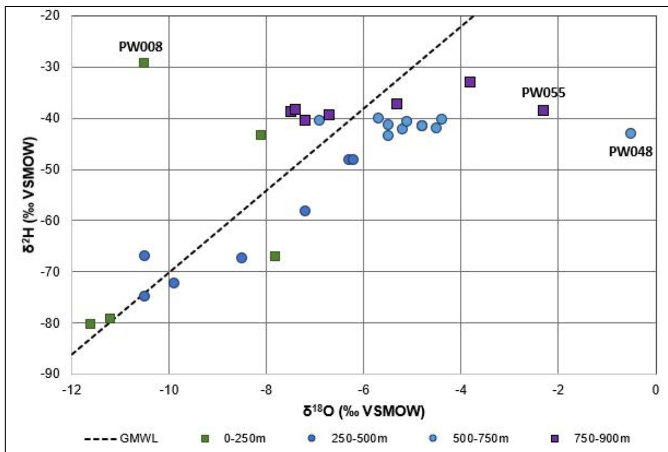
**Figure 6**  $^{18}\text{O}$ - $^2\text{H}$  Cross Plot, SB\_BH01 Porewater Samples. Samples SB\_BH01\_PW048 and SB\_BH01\_PW055 were noted to have low water content (<0.1% and 0.2%, respectively). Subsamples of SB\_BH01 PW055 were combined to have sufficient volume for analysis.
