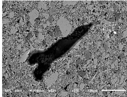
Location B: Black particles in the silty detrital-mineral matrix are organic fragments. Note the precipitated salts in the upper right.
