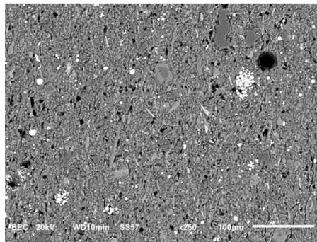
Location A: Fine-grained disseminated euhedral and framboidal pyrite in shale matrix. Typical of the entire section area.
