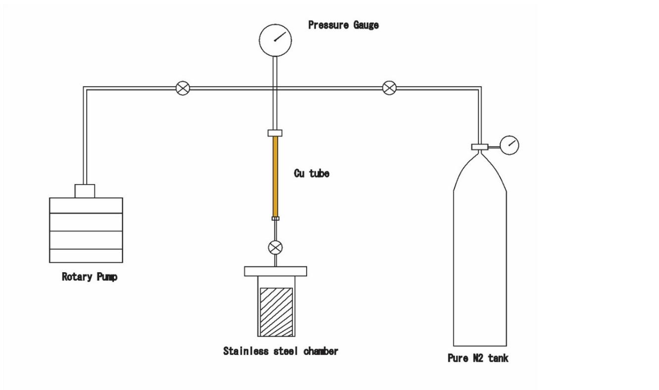
**Figure 2** Schematic for noble gas core sample encapsulation (Source: University of Ottawa, Noble Gas Isotope Laboratory)
