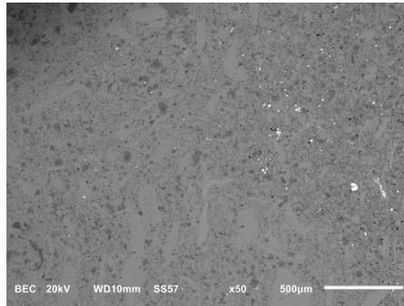
Location A: Micritic matrix to bioclasts. Dominantly calcite with disseminated dolomite (dark grey), pyrite (white), and organics (black).
