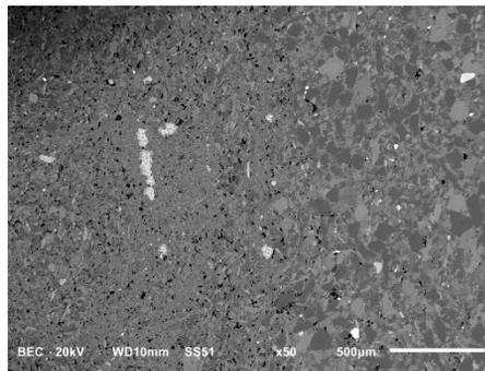
Location B: Boundary between fine-grained shale (left) and silty layer (right). Light grey linearly aligned grains in the centre-left are precipitates from dried porewater.
