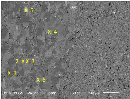
Location B: Carbonate cemented silty lens. Numbers indicate locations of EDS analyses used to identify minerals 1) quartz, 2) dolomite, 3) dolomite (ferroan), 4) calcite, 5) apatite, 6) calcite.
