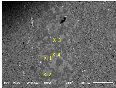
Location A: Silty lens. Numbers indicate locations of EDS analyses used to identify minerals 1) quartz, 2) calcite, 3) dolomite, 4) dolomite.
