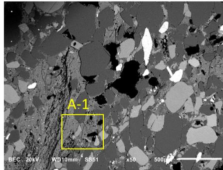
Location A: Rounded detrital grains of quartz (dark grey) K-feldspar (medium grey) and apatite (white). Black organic material fills pores.
