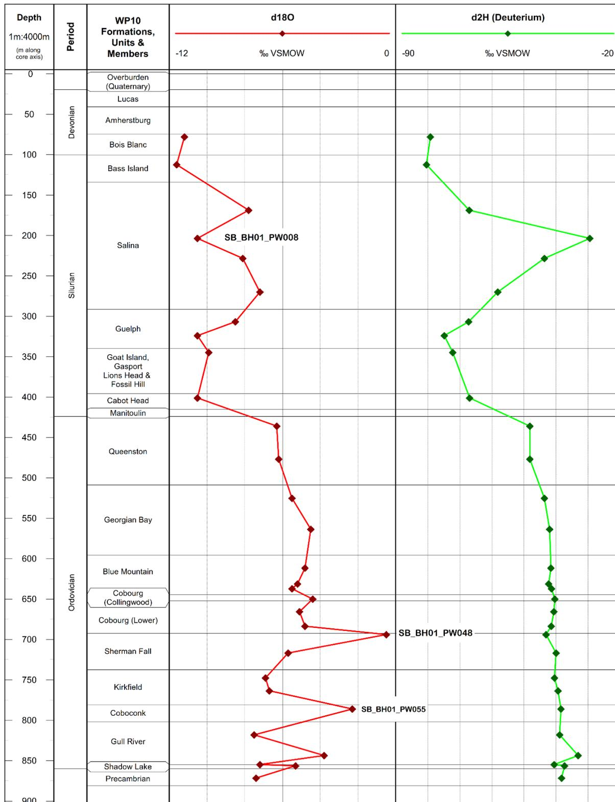
**Figure 7** Profile of  $\delta^{18}\text{O}$  and  $\delta^2\text{H}$  (Deuterium) of Porewater, SB\_BH01 Core Samples. Samples SB\_BH01\_PW048 and SB\_BH01\_PW055 were noted to have low water content (<0.1% and 0.2%, respectively). Subsamples of SB\_BH01 PW055 were combined to have sufficient volume for analysis.
