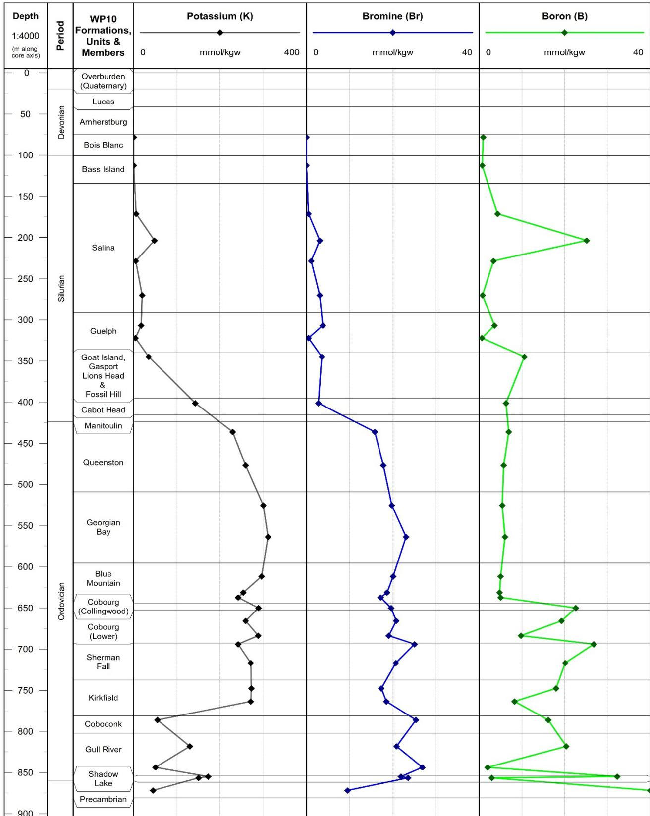
**Figure 5 Profile of Potassium, Bromine, and Boron Strontium Concentrations in Porewater from Vacuum Distillation, SB\_BH01 Core Samples**
