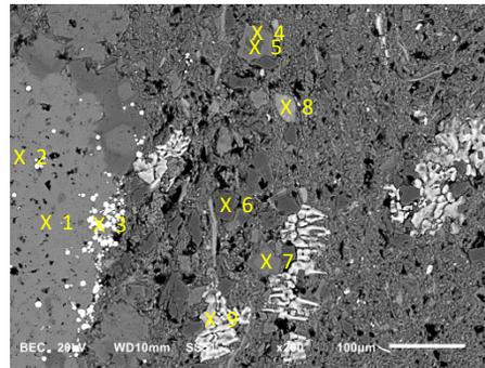
Inset A-1: Higher magnification image from inset shown in A. A calcite fragment is along the left margin, black interstitial material is organic and the large light-grey regions are NaCl precipitates from dried porewater. Numbers indicate locations of EDS analyses used to identify minerals 1) calcite, 2) calcite, 3) pyrite, 4) dolomite (ferroan), 5) dolomite, 6) quartz, 7) dolomite (ferroan), 8) Fe-Mg-Al-silicate, 9) NaCl precipitate from dried porewater.
