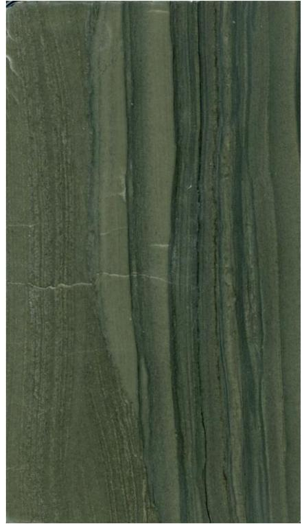
SB\_BH01\_PW013 Salina A2 Carbonate
