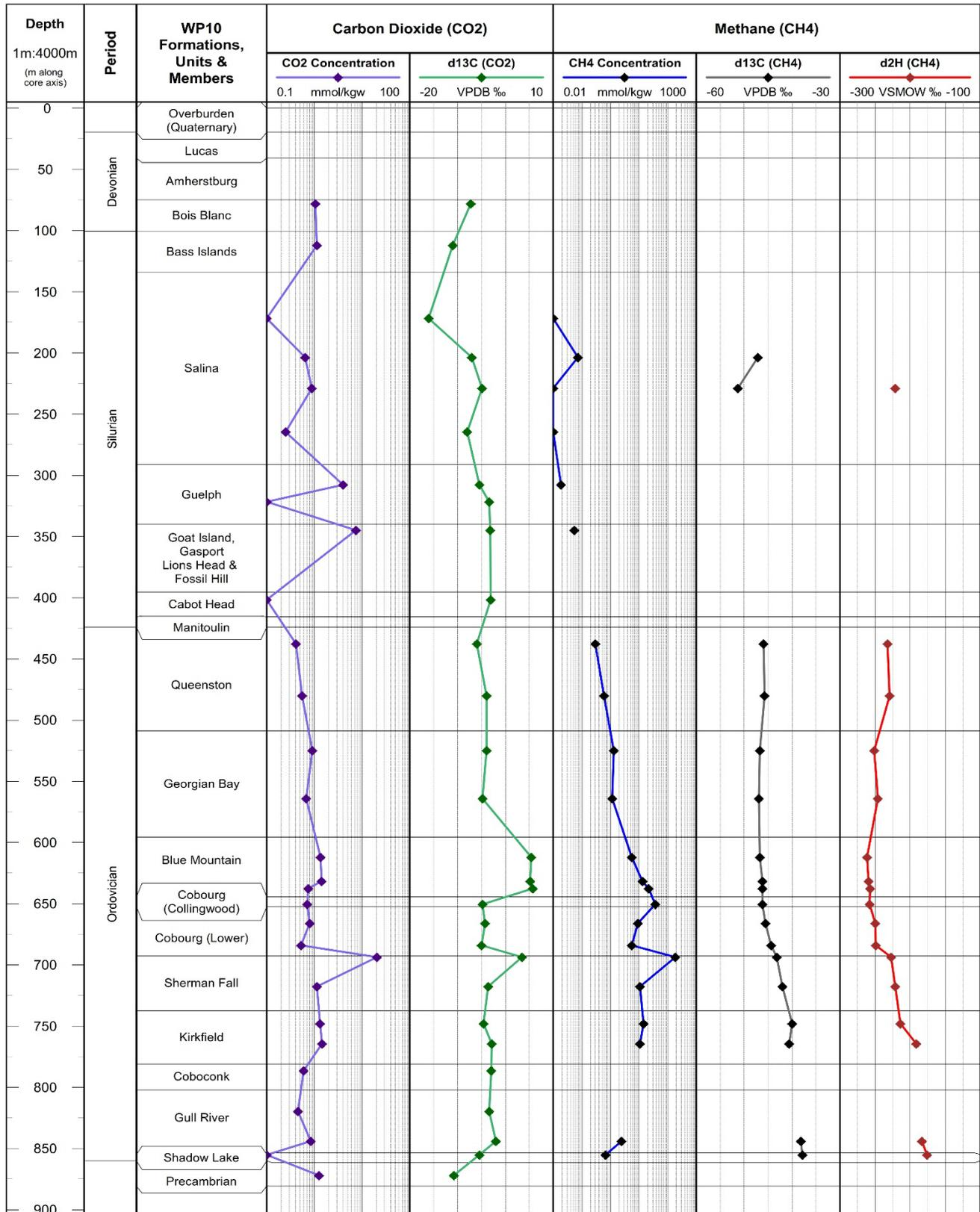
**Figure 10 Profile of Methane and Carbon Dioxide Concentrations and Isotopes from SB\_BH01 Core Samples**
