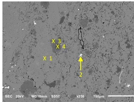
Location A: dominantly calcite with disseminated dolomite and pyrite, and organics (black) infilling pore spaces. Numbers indicate locations of EDS analyses used to identify minerals 1) calcite, 2) pyrite, 3) dolomite (ferroan), 4) dolomite.
