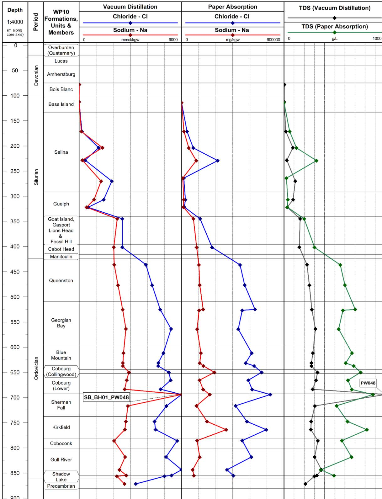
**Figure 3 Profile of Chloride, Sodium, and TDS Concentrations of Porewater from Vacuum Distillation and Paper Absorption, SB\_BH01 Core Samples.** TDS calculated assuming freshwater density (1000 kg/m<sup>3</sup>). Sample SB\_BH01\_PW048 was noted to have exceptionally low water content and strong degassing during sampling.
