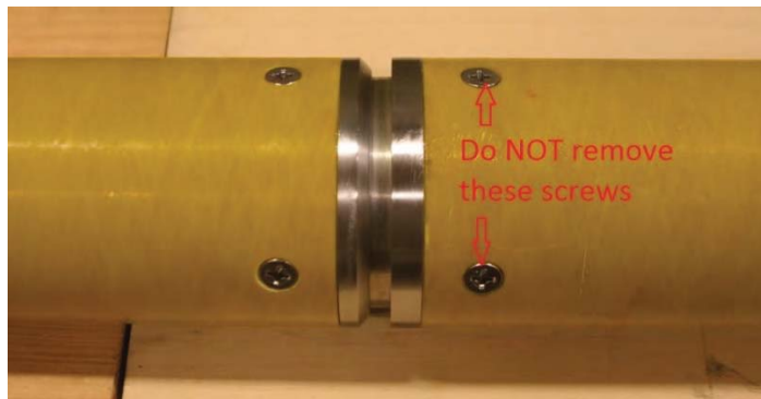
Figure 28: Completely assembled Double Joint. Use Phillips Machine Screws, #1/4-20 x 5/8". For disassembly, do not remove the screws on the "downhole" side of this or any of the Double Joints.
