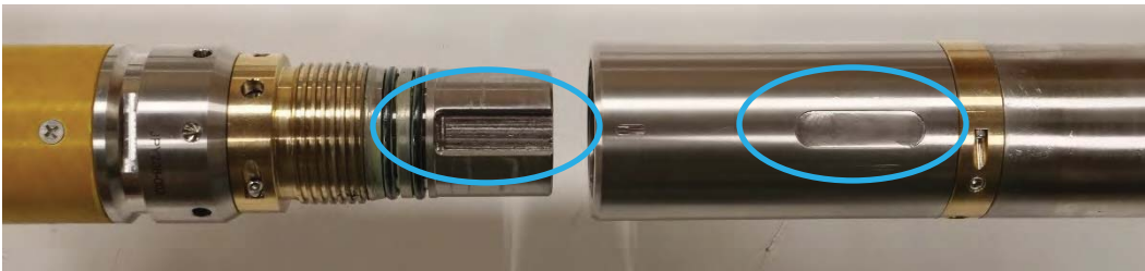
Figure 18: Proper alignment of the Field Joints of the Javelin Slim – the dimpled markings on the two sides of the joint (circled) should be aligned with one another.
