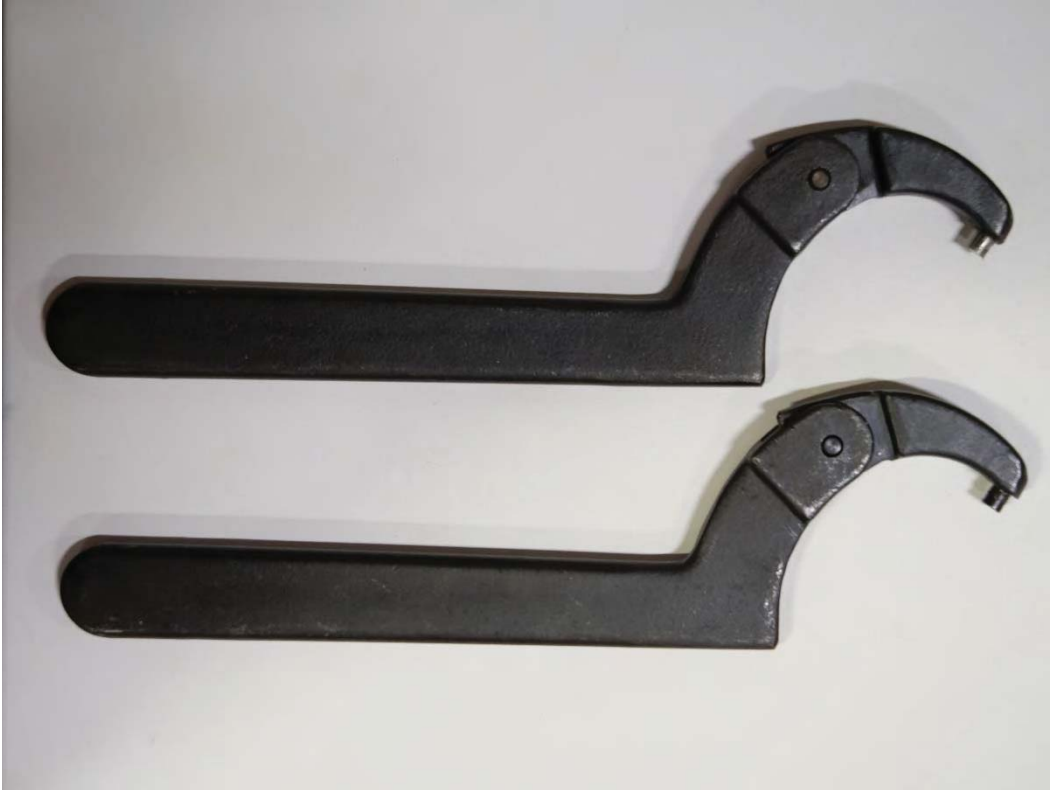
Figure 17: Adjustable spanner wrenches for tightening and loosening Field Joints. One pin may be slightly smaller to fit smaller tightening divots on Field Joint.
