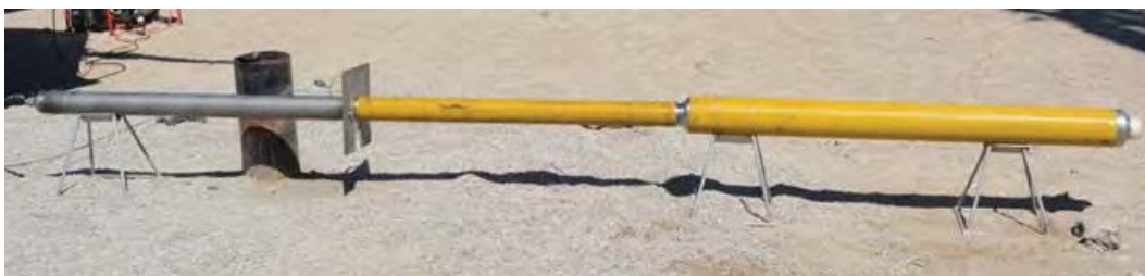
Figure 34: Assembled three-section Javelin Wireline Tool with JPX525F Analog MR Probe.
