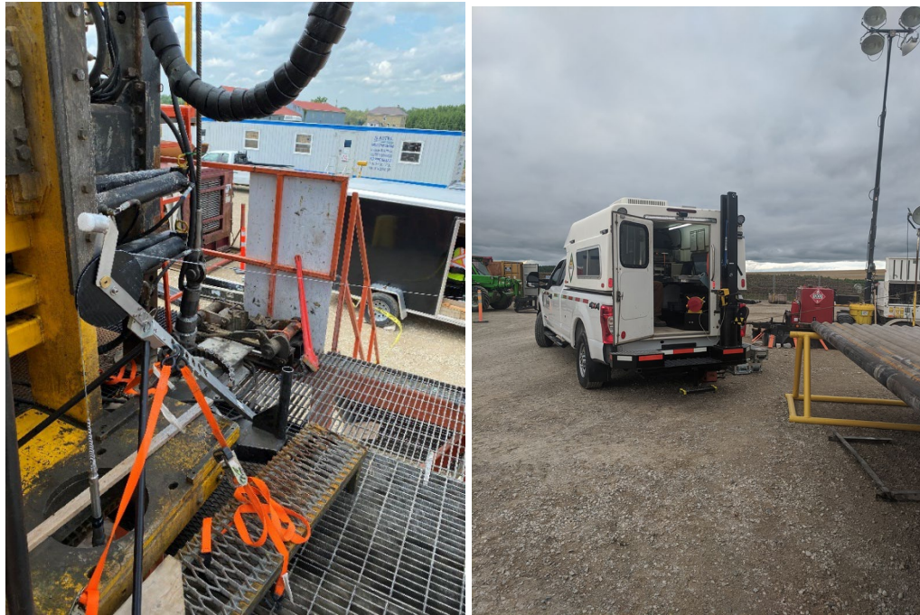
Figure 3 Field Equipment Setup Phase 1: Winchline extended from field office trailer over pulley on drill floor to “zero” at surface reference. Phase 2: Winchline extended from Colog truck.
