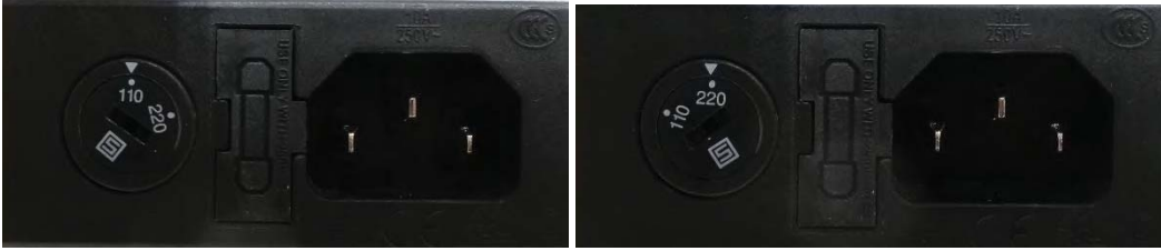
Figure 11: Power input to Surface Station configured for 110V/60Hz (left) and 220V/50Hz (right).
