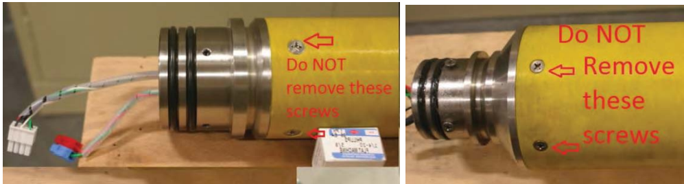
Figure 24: Double Joint on the uphole side of the JPX350F (left) and JPX525F (right). Each of these joints connects to the Power Module.
