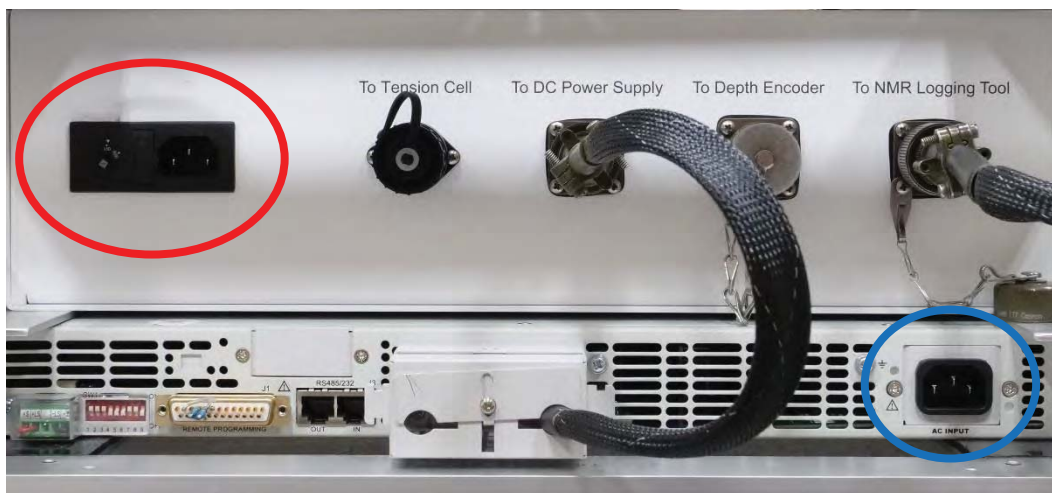
Figure 10: Rear view of the Surface Station (upper unit) and power supply (lower unit), showing C13-style power inputs (circled). The Surface Station power input (red circle) requires user configuration to select between 110V and 220V. The power supply power input (blue circle) can accept 110V/60Hz and 220V/50Hz without user configuration.
