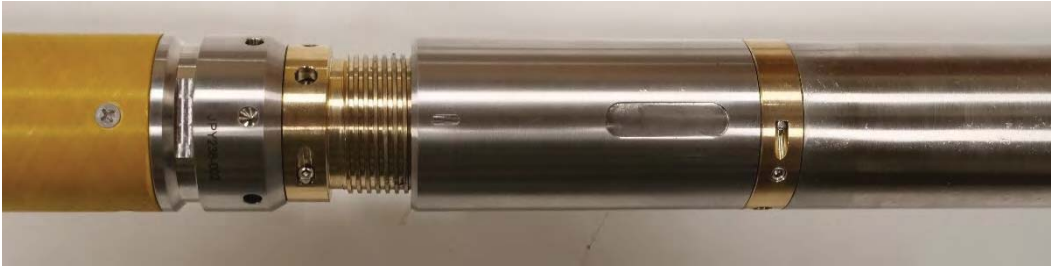
Figure 19: Insert the two sections of the tool together until reaching this point—O-rings are completely inside the field joint, and the brass threads are just touching the uphole side of the Field Joint.
