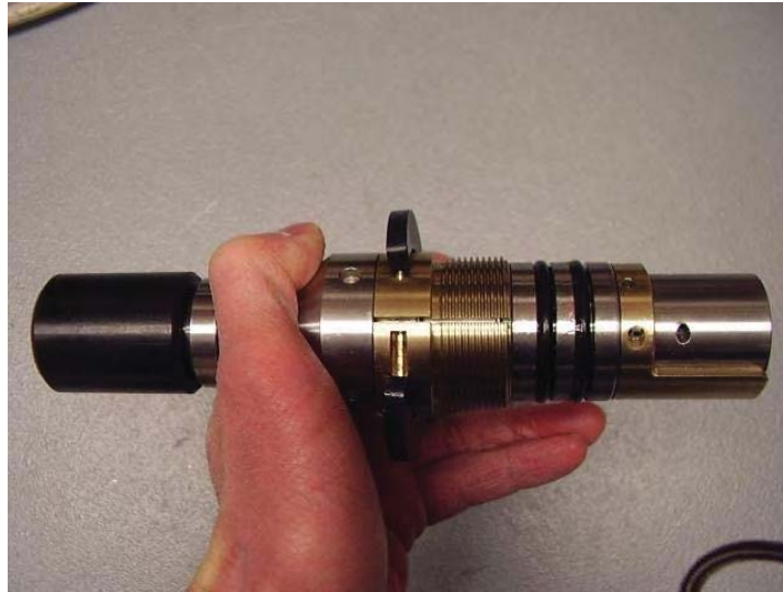
Figure 6-1 Disassembly of the threaded ring
