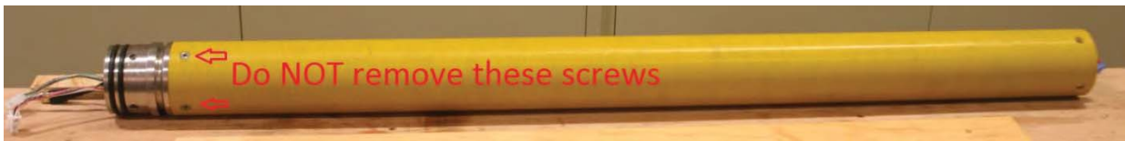
Figure 6: Power Module of Javelin Max (3-Section).
