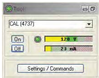
Figure 4-12 Nominal power consumption when calliper motor does not operate
