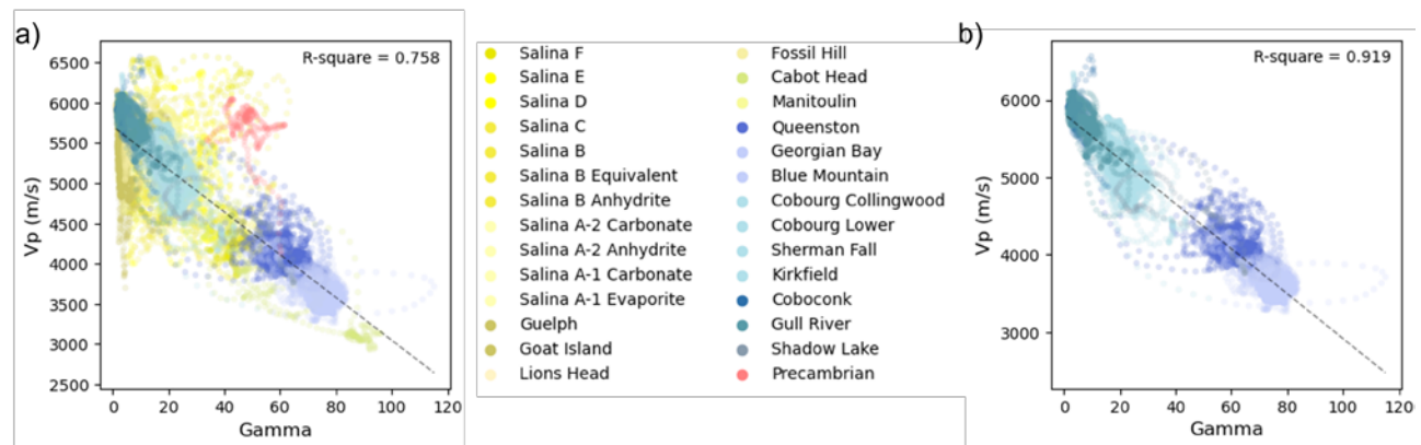
Figure 8. Correlation between P-wave velocity versus natural gamma. a) shows results for all formations logged in SB_BH01 with an R-squared coefficient of correlation of 0.76. b) presents results for Ordovician formations which significantly improving the correlation coefficient to 0.92.
