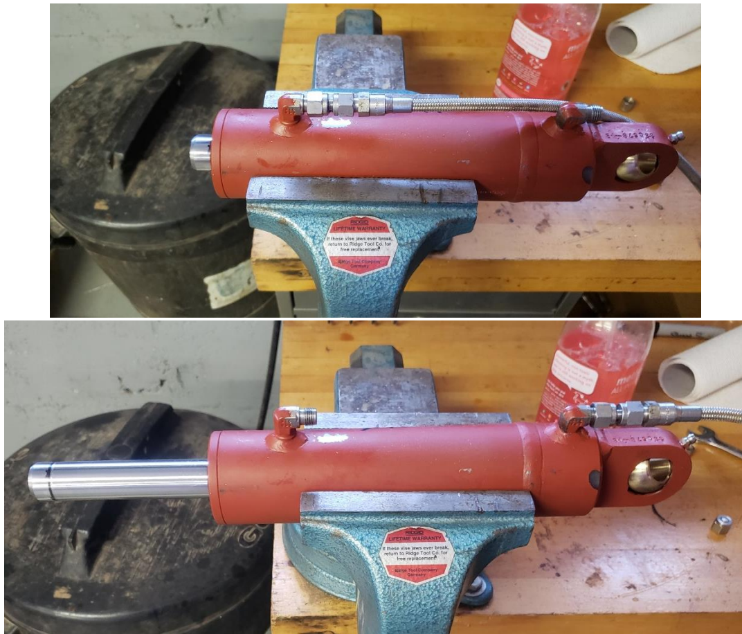
Figure 2.7 Hydraulic Pulse Generating Piston.
