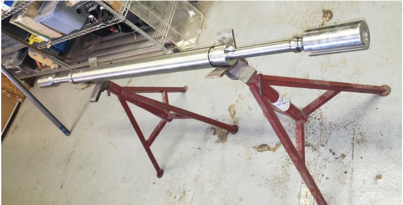
Figure 2.6 Downhole Shut-In Valve (DHSIV).
