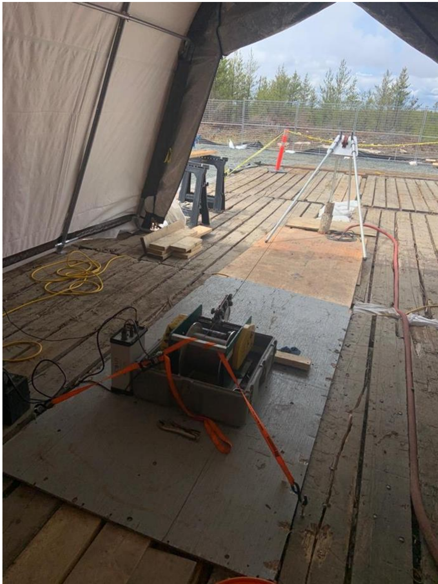
Figure 3: Winch bolted to ground and setup for IG_BH05.
