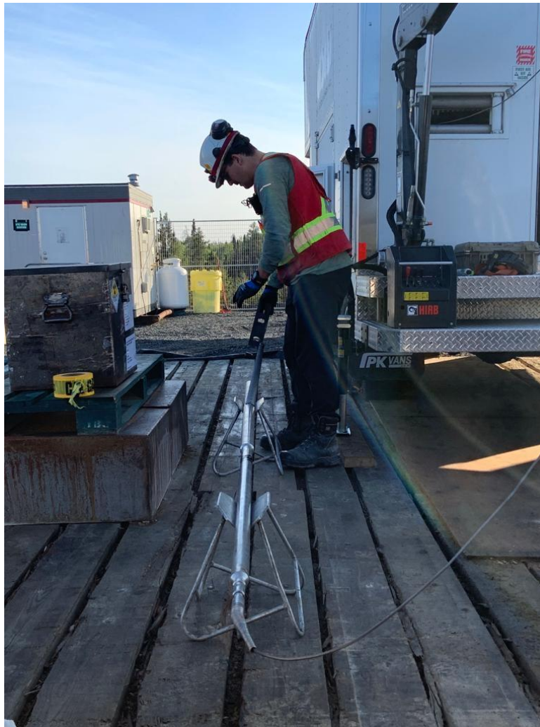
Figure 6: DGI setup for borehole logging
