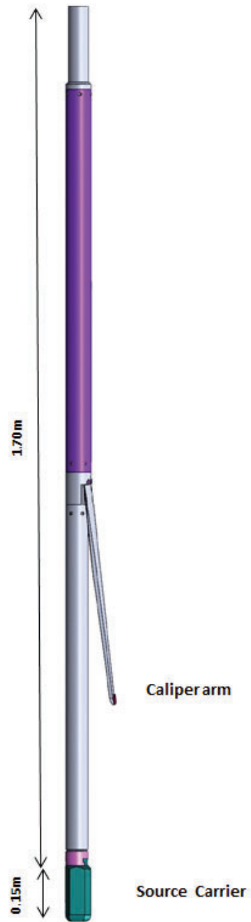
Figure 1-1 Tool general arrangement
