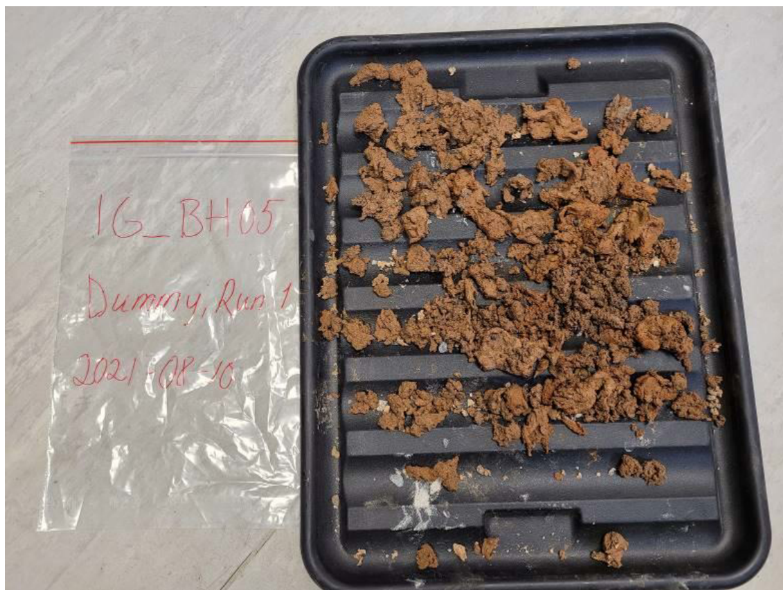
Figure 5-2. Content of dummy probe after the first run in IG_BH05.
