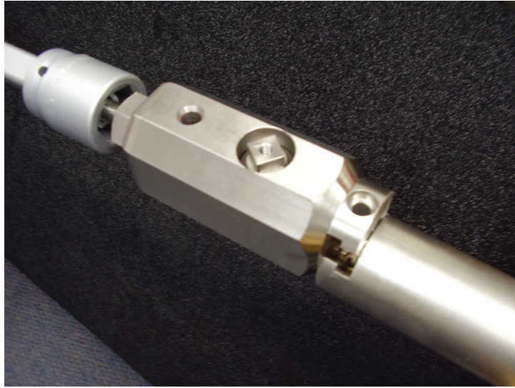
Figure 3-15 Installing Source Carrier onto probe with Source Handling Tool
