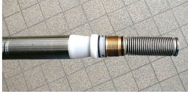
Figure 6-8 Bellows cover removed
