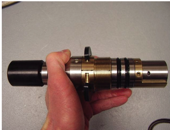
Figure 5-1 Disassembly of the treaded ring
