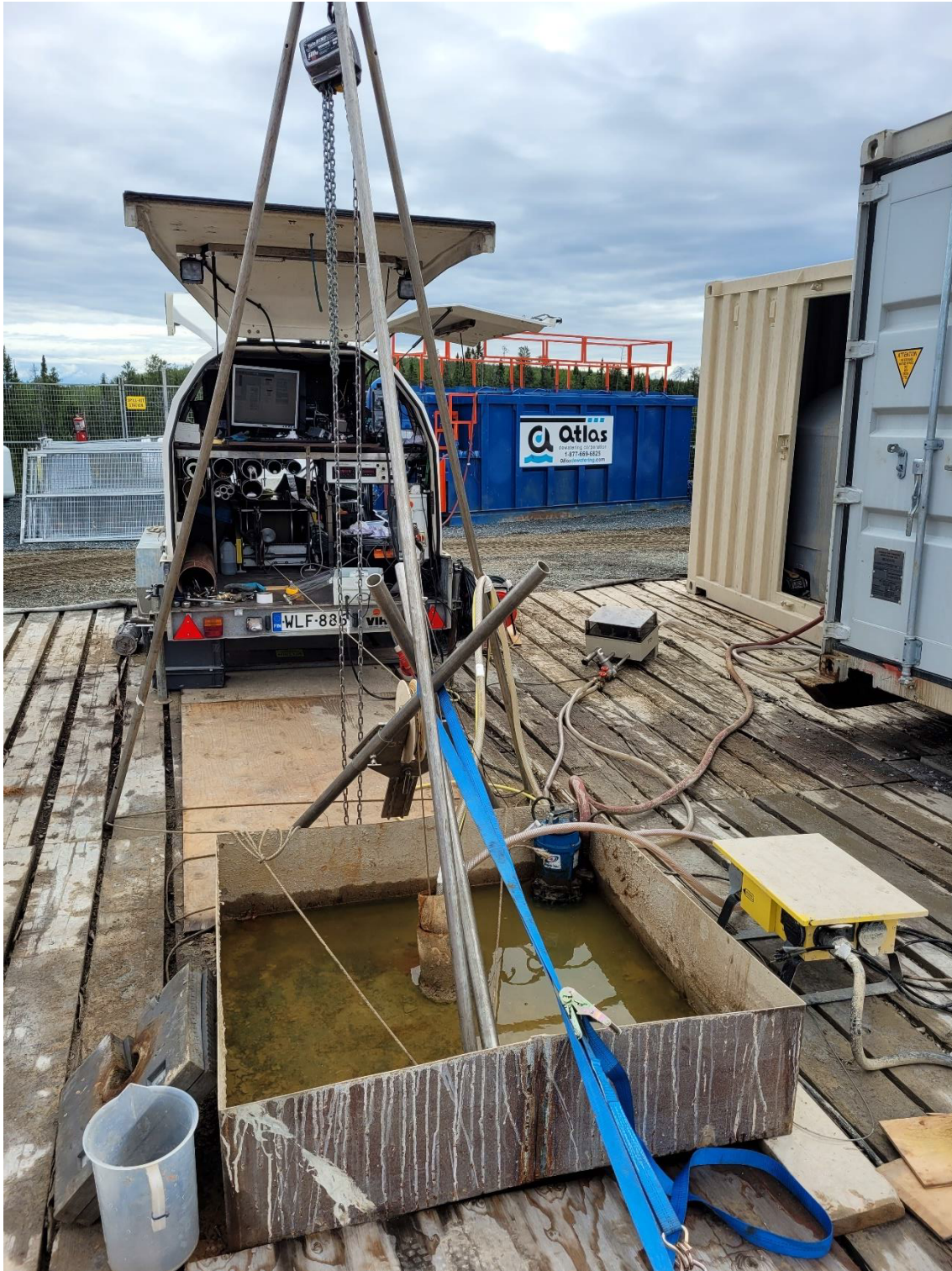
Figure 1-2. Borehole IG_BH05 and PFL measurement equipment..
