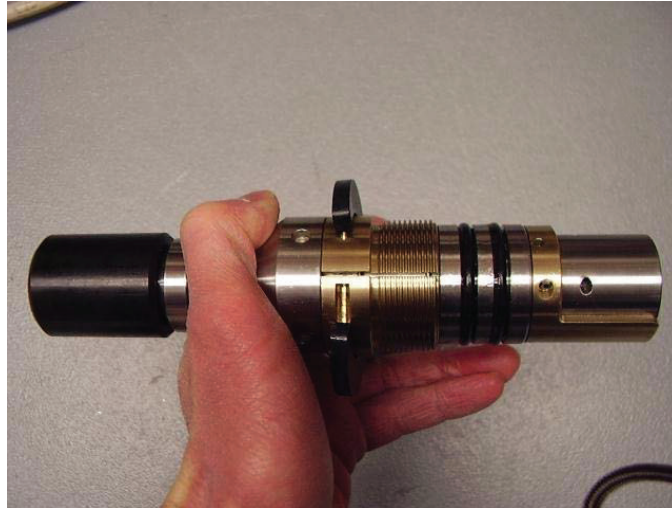
Figure 6-1 Disassembly of the treaded ring
