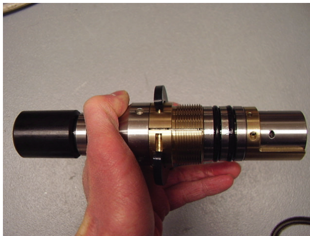
Figure 6-2 Disassembly of the locking ring –step 1
