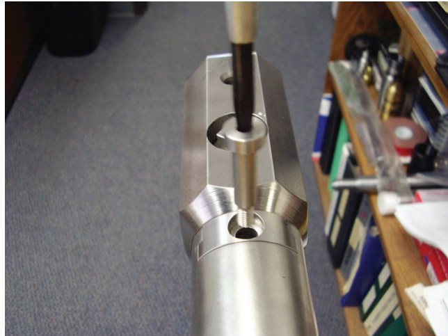
Figure 3-16 Inserting locking screw into the Source Carrier
