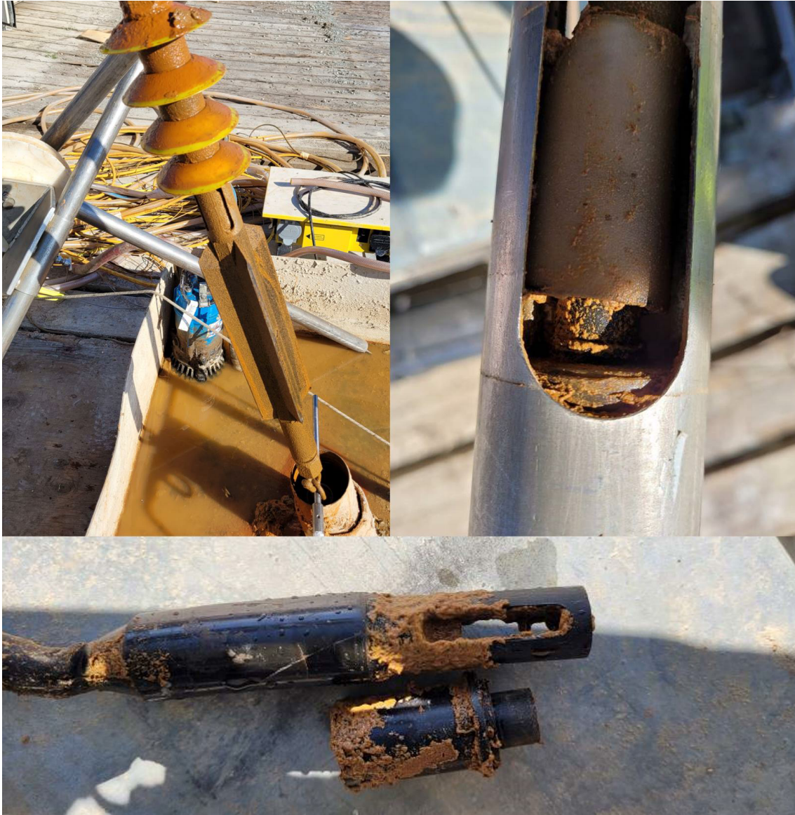
Figure 7-2. Dirt coating at PFL probe after flow logging run 2.
