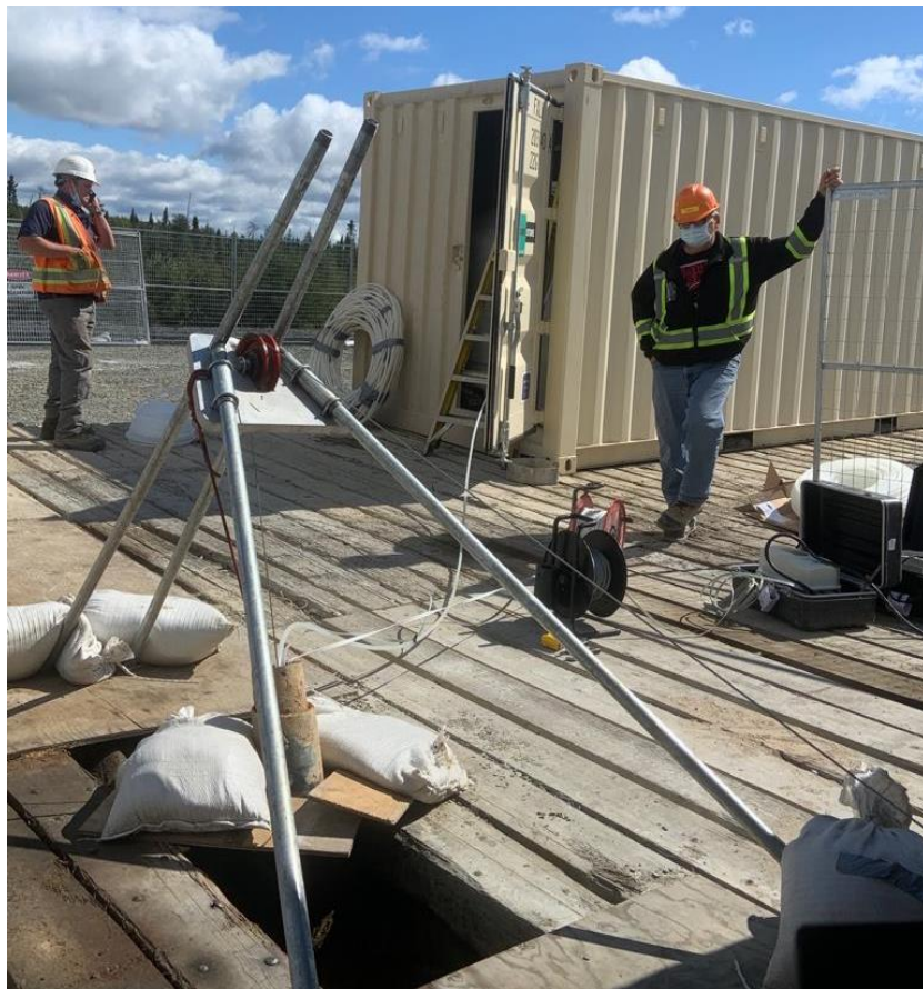
Figure 5: Borehole wireline tripod and wheel
