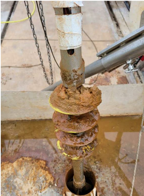
Figure 7-1. PFL probe upped rubber disks after flow logging.
