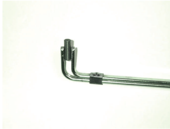
Figure 3-8 Detail of source in tongs
