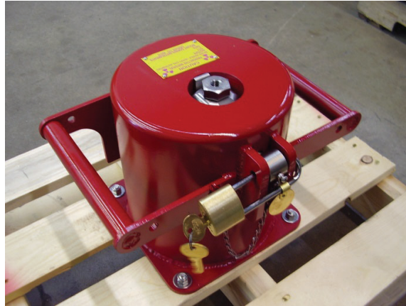
Figure 3-14 Shield with source and source carrier installed
