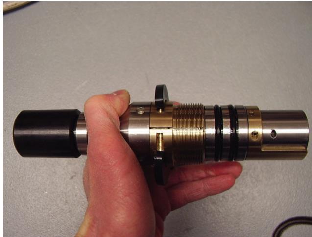
Figure 6-2 Disassembly of the locking ring –step 1
