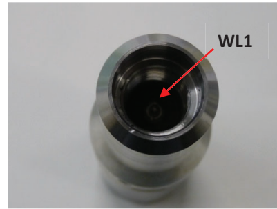
Figure 9-4 MSI top connection to cable head
