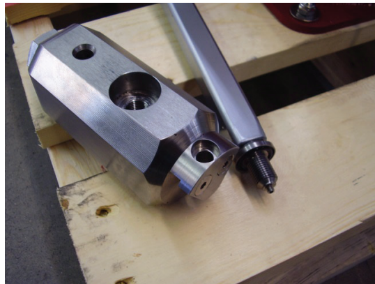
Figure 3-9 Source Holder, Source Installation Tool, and Retainer Screw
