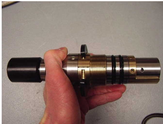
Figure 5-1 Disassembly of the treaded ring
