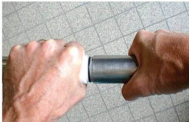
Figure 6-7 Unscrewing the bellows cover
