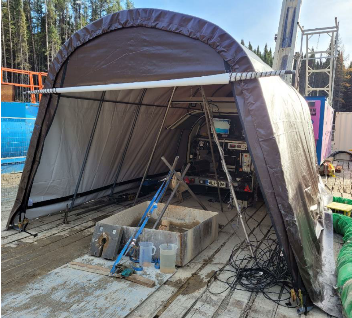
Figure 1-2. Borehole IG_BH06 and PFL measurement equipment.
