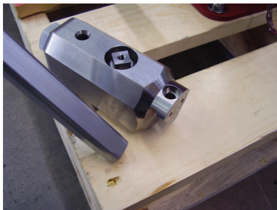
Figure 3-12 Source carrier with Source Installed
