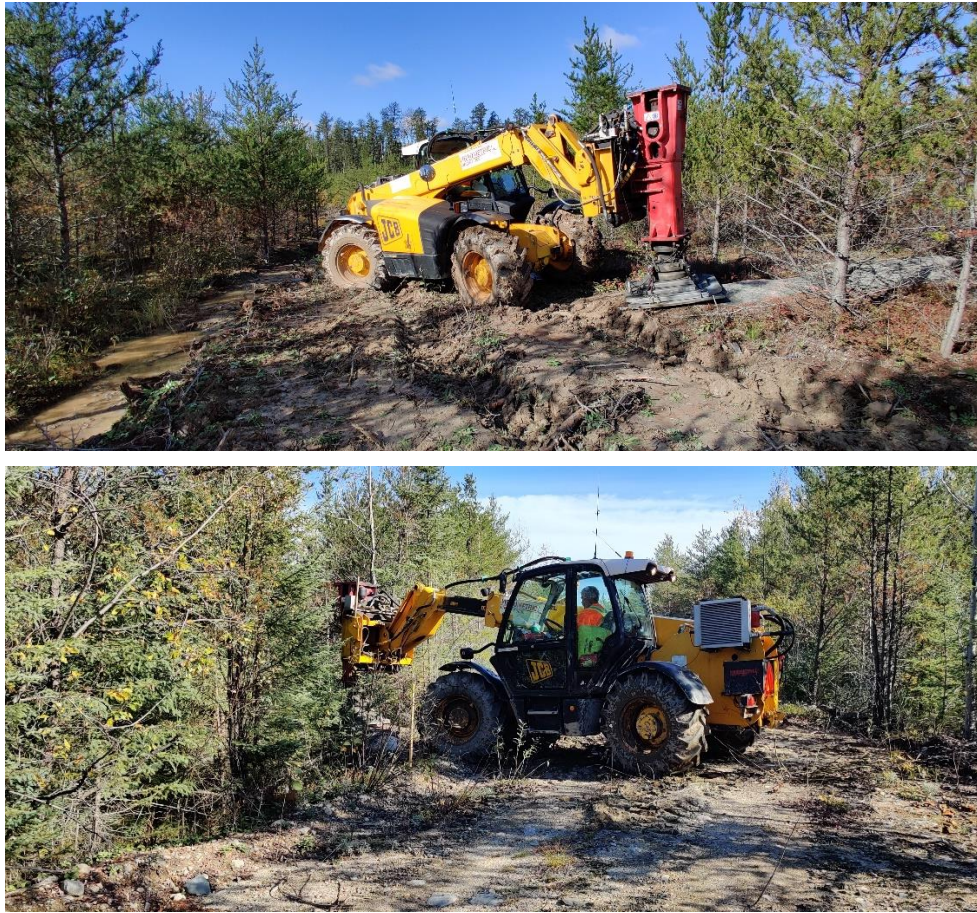
Figure 3: The VIBSIST-3000 seismic source used for the VSP survey in IG_BH05. A thick rubber mat was used for the source, in order to avoid direct contact with outcrops.
