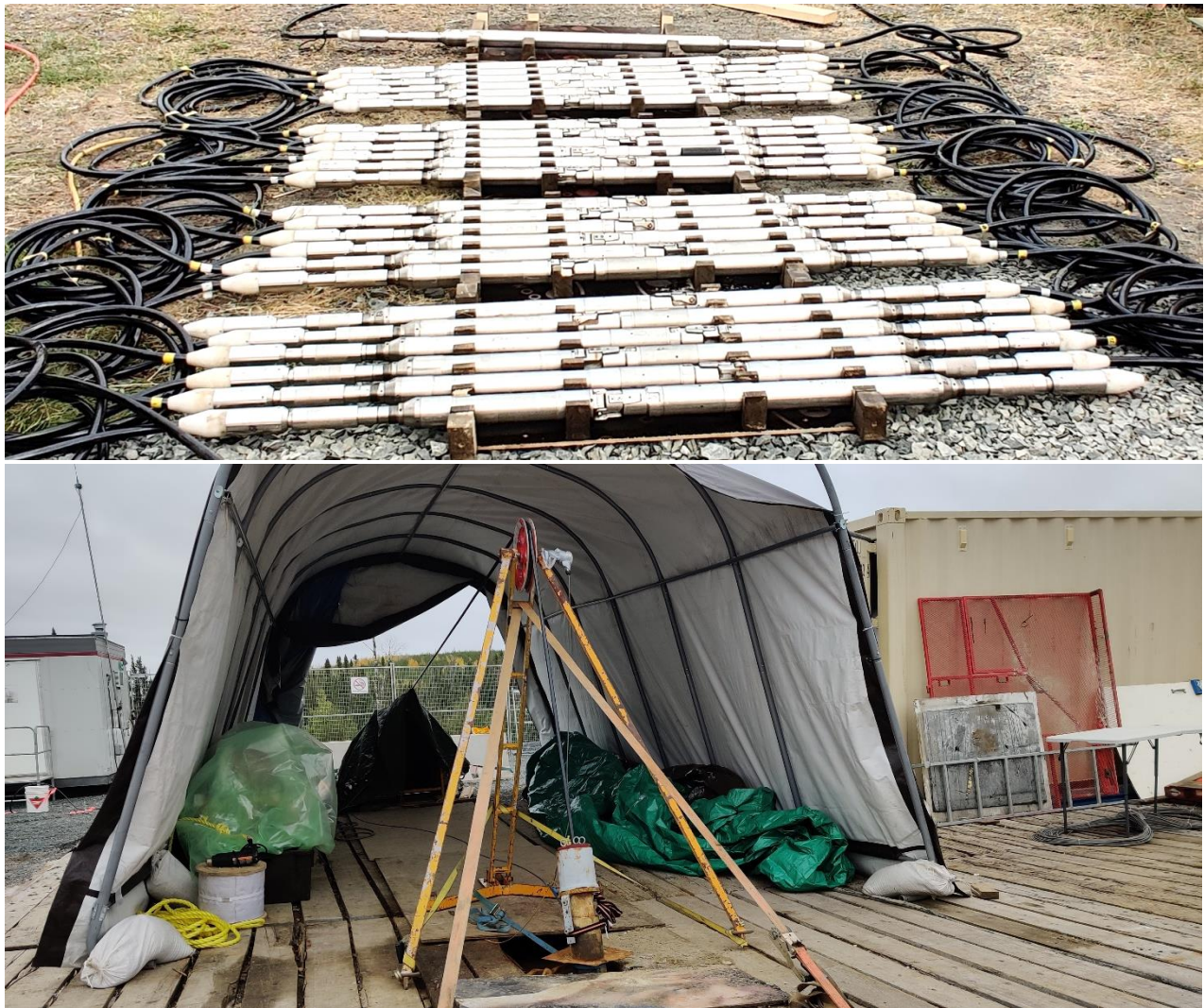
Figure 4: Detail of the 3-component modules with clamping arms for the RD-XYZH geophone receiver system and picture of the receiver cable winch, together with the acquisition setup at borehole IG_BH05.
