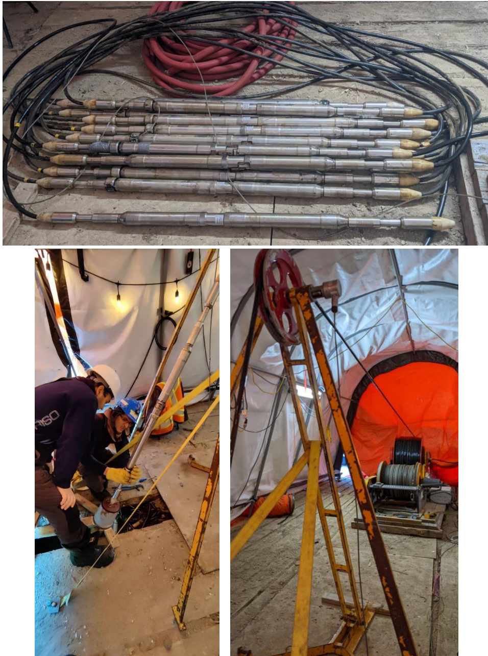
Figure 4: Detail of the 3-component modules with clamping arms for the RD-XYZH geophone receiver system and pictures of the receiver installation and cable winch. Acquisition setup at borehole IG_BH06.
