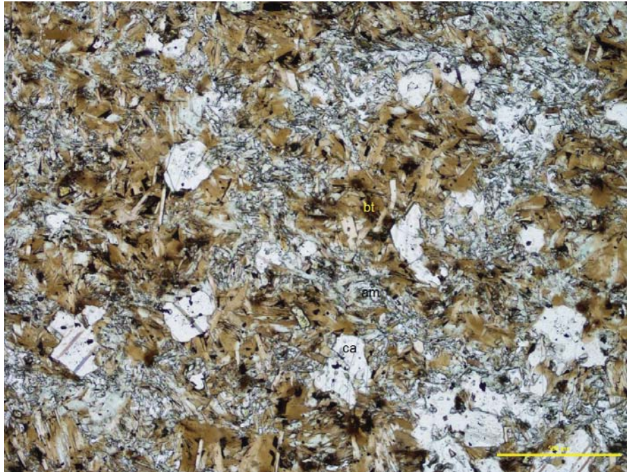
Figure 43 Porphyroblasts of calcite (ca) and irregular clusters of biotite (bt) are associated with fine-grained crystals of amphibole (am) and quartz. Crossed polarizers transmitted light.
