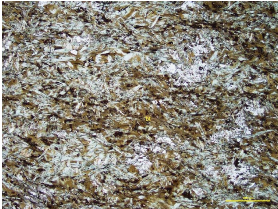
Figure 48 The biotite (bt) tends to form slightly elongate crystal clusters, in which the biotite flakes and lamellae are randomly oriented, and define a weak schistosity. Plane polarized transmitted light.
