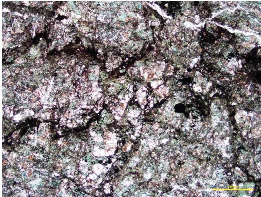
Figure 58 The fine-grained anhedral mineral aggregate is brecciated (crackle breccia), and it is filled in by irregular veinlets of iron oxides (opaque) and calcite (white). Plane polarized transmitted light.
