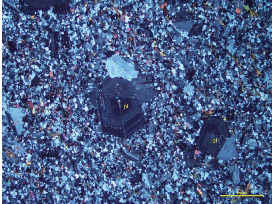
Figure 32 Subhedral crystals of plagioclase (pl) show euhedral growth zoning and are immersed within a weakly schistose matrix of quartz and biotite. Crossed polarizers transmitted light.
