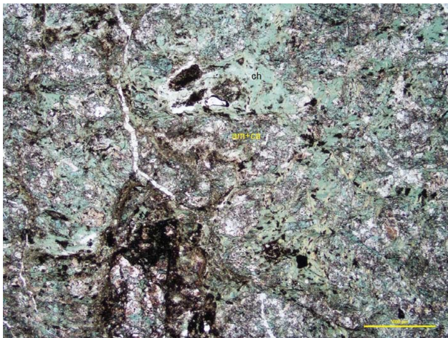
Figure 59 Irregular clusters of chlorite (ch) are intergrown with the amphibole and the calcite (am+ca). Plane polarized transmitted light.
