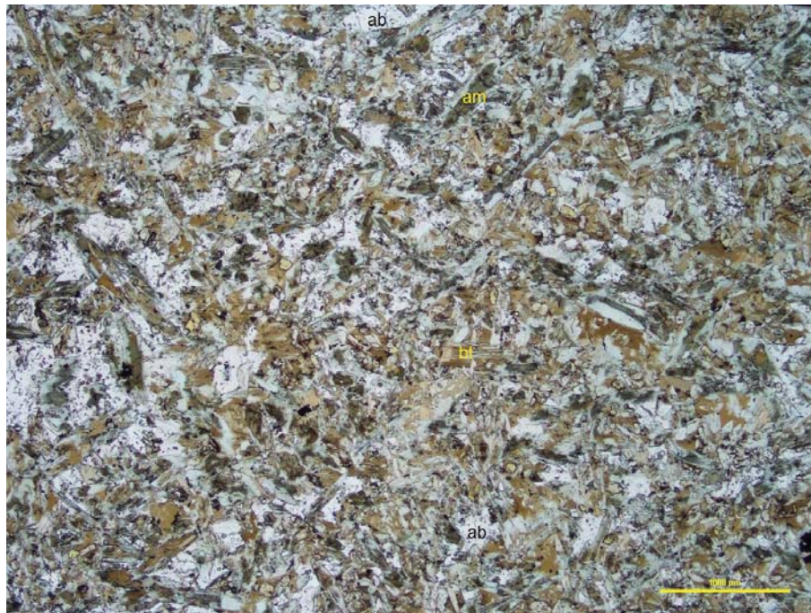
Figure 47 Xenoblastic crystals of albite (ab) are intergrown with randomly oriented prisms of amphibole (am), xenoblastic crystals of biotite (bt), and subordinate calcite and epidote, all of which define a heterogeneous isotropic microstructure. Plane polarized transmitted light.
