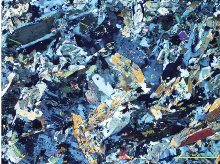
Figure 51 Xenoblastic and randomly oriented crystals of plagioclase (pl), amphibole (am), and biotite define a granular and isotropic microstructure. Crossed Nicols transmitted light.
