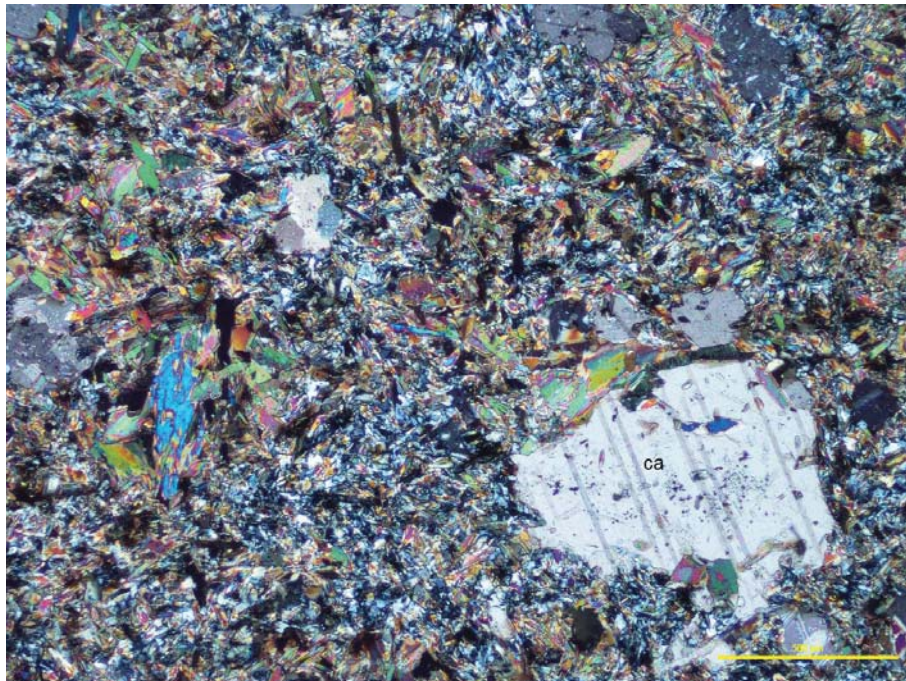
Figure 44 Xenoblastic crystals of calcite overprinted the weakly foliated microstructure defined by biotite, amphibole, and quartz. Crossed polarizers transmitted light.
