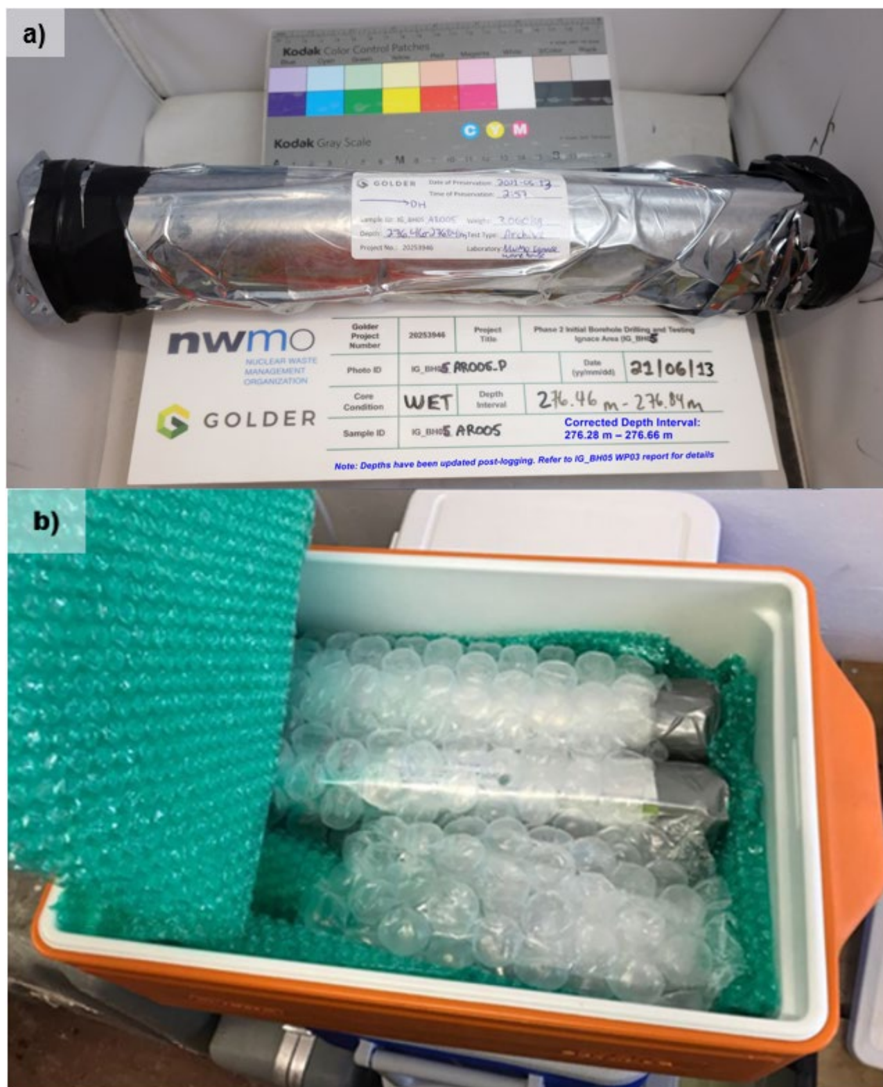
Figure 17 : Examples of Sample Preservation Methods: a) Example Photograph of a Preserved Archive (AR) Rock Core Sample (IG_BH05_AR005), b) Example Photograph of Preserved Rock Core Samples ready for Laboratory Shipment
