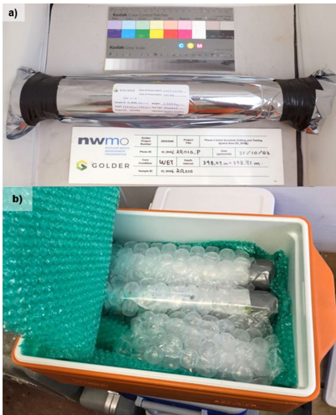
Figure 17 : Examples of Sample Preservation Methods: a) Example Photograph of a Preserved Archive (AR) Rock Core Sample (IG_BH06_AR010), b) Example Photograph of Preserved Rock Core Samples ready for Laboratory Shipment
