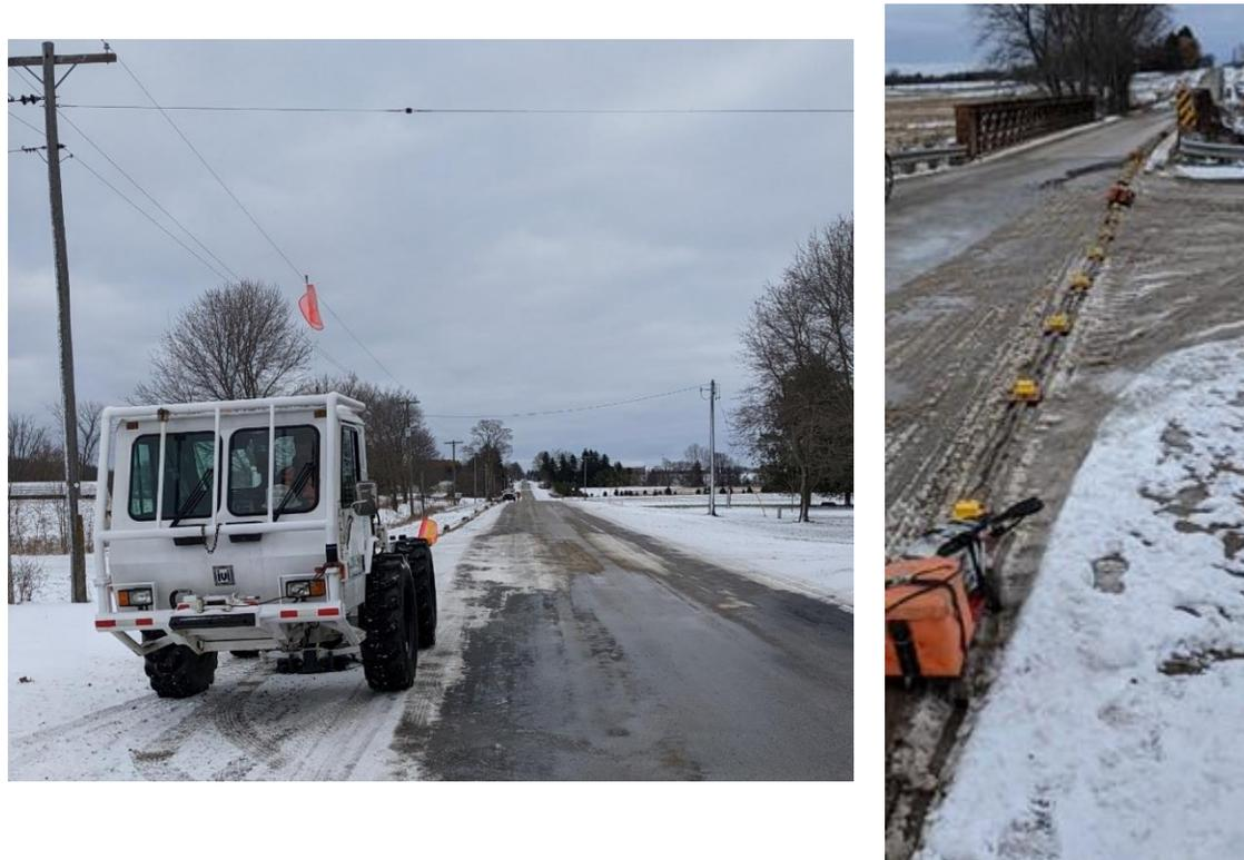
**Figure 2 2D seismic data acquisition equipment. Left: Vibroseis unit and geophone streamer; Right: Detailed view of land streamer equipment (geophones are yellow)**
