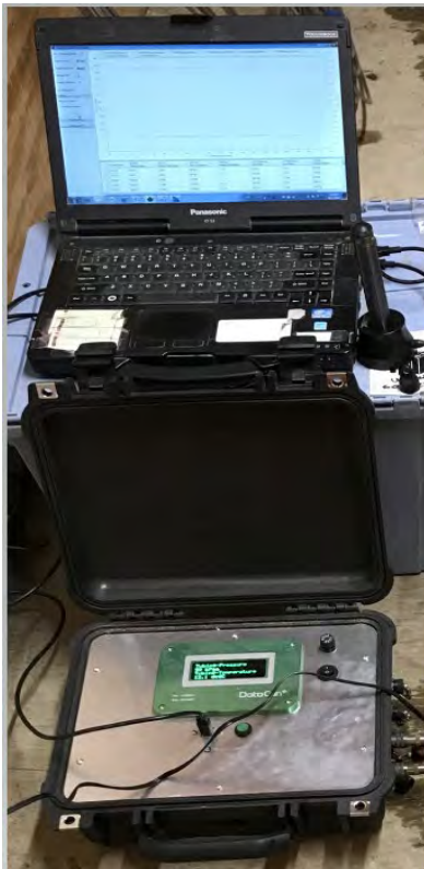
Figure 3: DataCan Surface Readout Box, Model 105421
