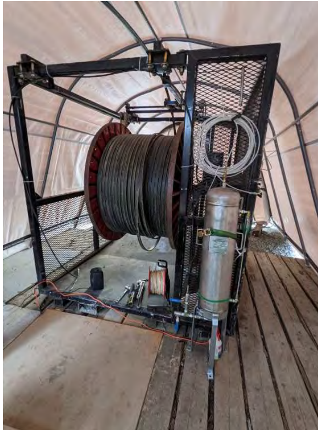
Figure 6: Work area tent with flatpack and pressure vessel (packer inflation manifold with pressure gauge on right side of cage) (see Figure 8)
