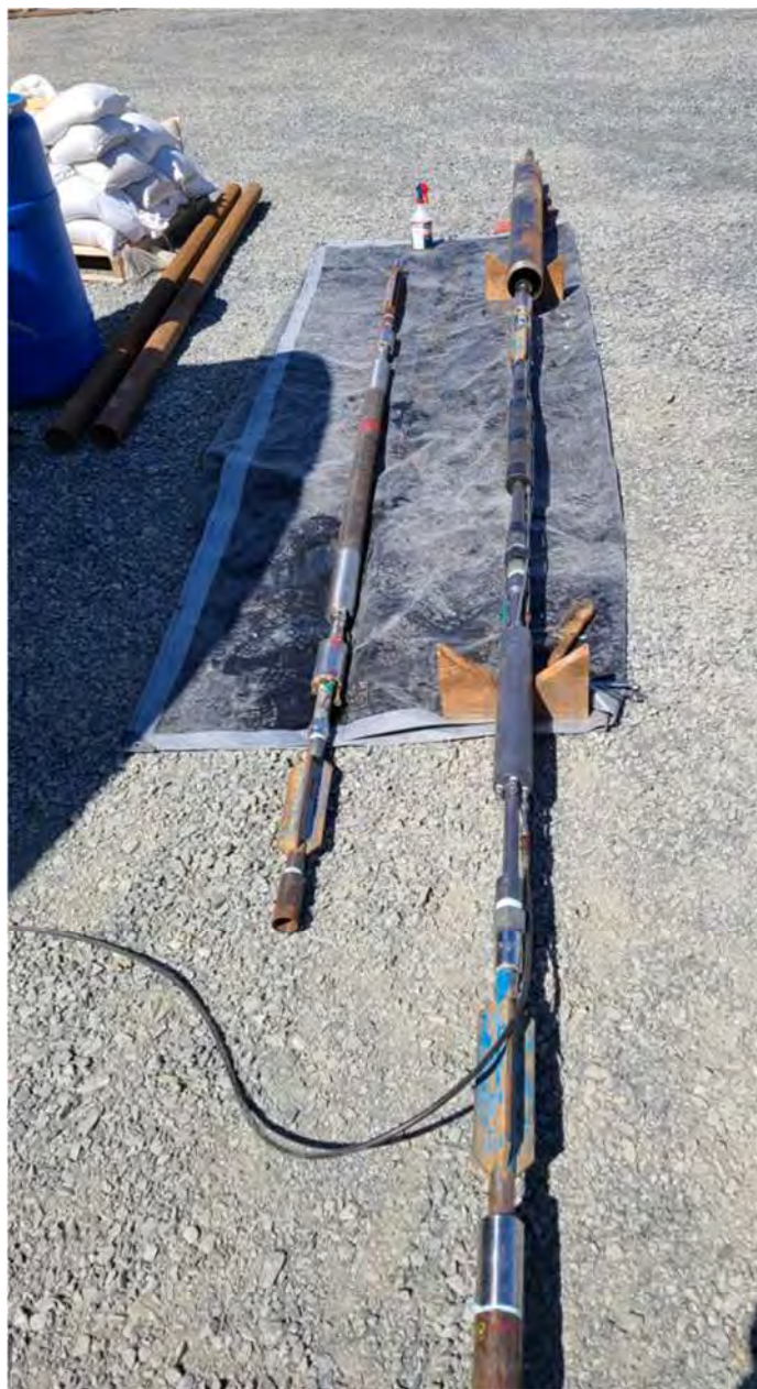
Photo 1 – Packer testing tool with lower packer shown on left. Datalogger, DHSIV and upper packer shown on right.
