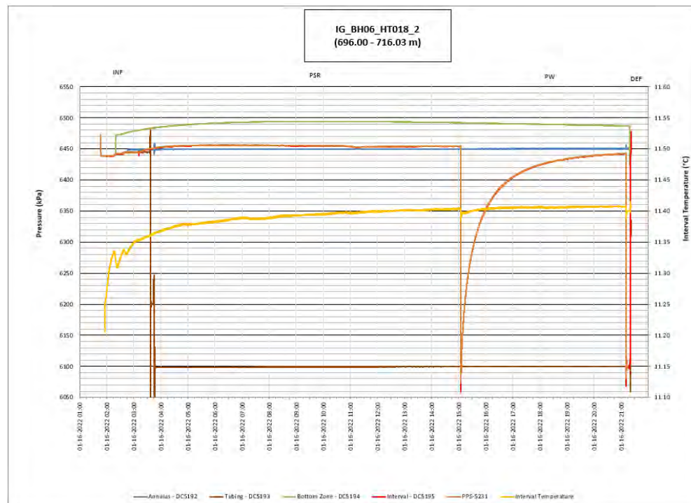
Figure 217: HT018_2 Annotated test plot showing monitored zone pressure and interval temperature.
