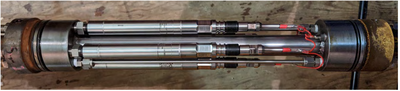
Figure 4: DataCan Gauge Carrier and Transducers with Outer Protective Casing Removed
