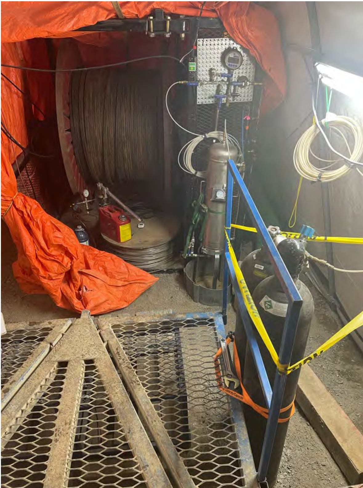
Photo 3 – Front of flatpack cage with DHSIV (red reservoir tank with hand pump below flatpack reel), nitrogen cylinders (foreground, lower right of photo), pressure vessel and manifold (to right of flatpack, in front of cage).
