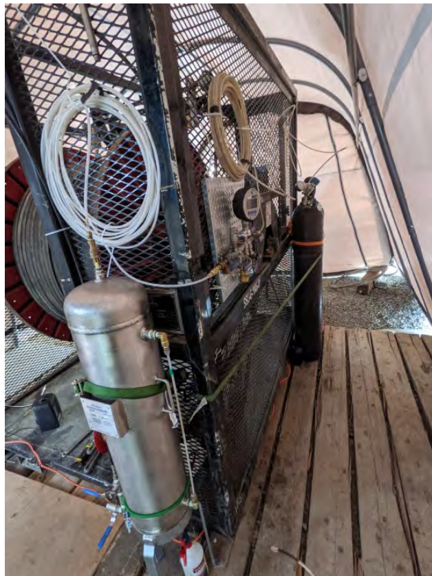
Figure 8: Pressure vessel (front) and packer inflation manifold with pressure gauge and nitrogen bottle on side of flatpack cage
