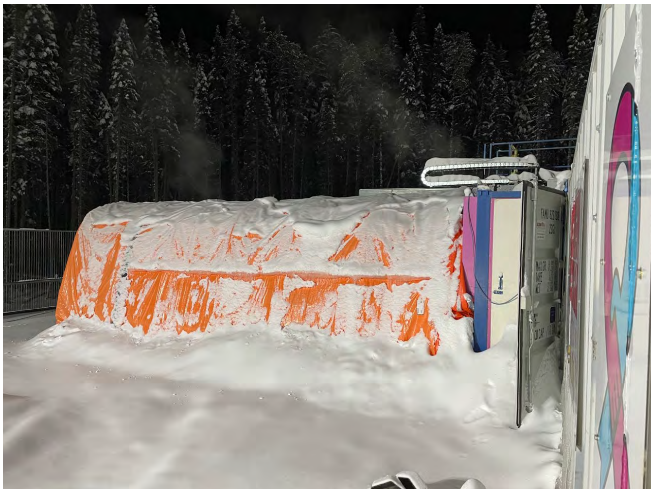
Photo 1 – Winterized enclosure for BH06 Hydraulic Testing shown from exterior.
