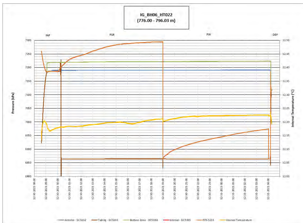
Figure 265: HT022 Annotated test plot showing monitored zone pressure and interval temperature.
