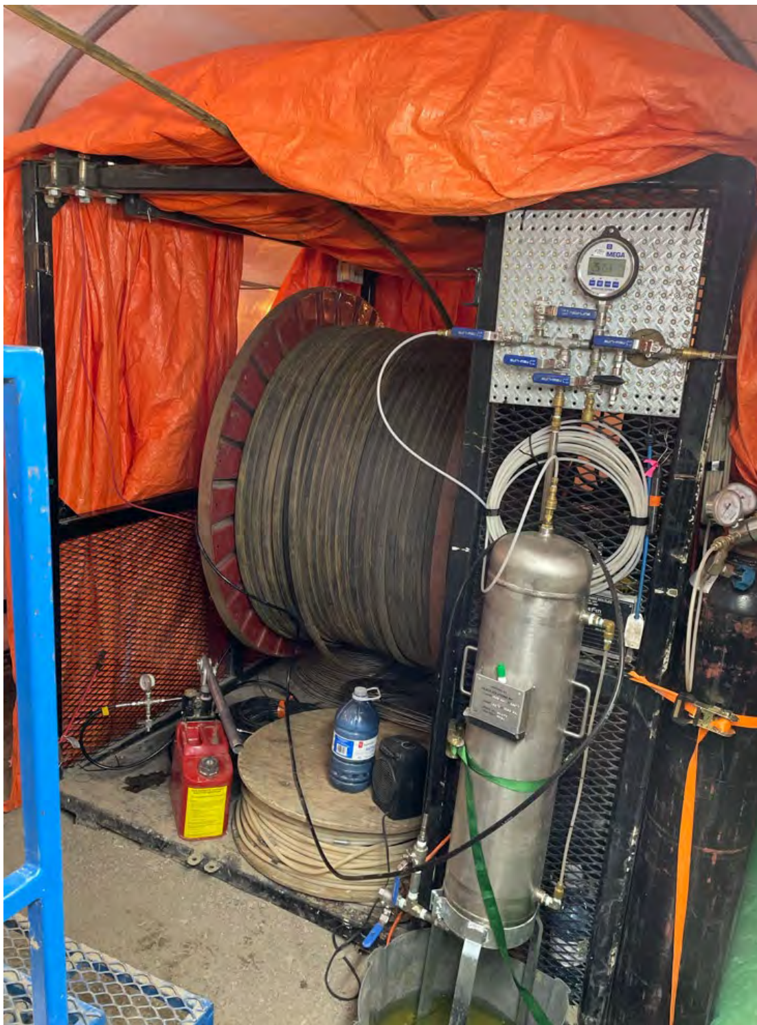
Photo 4 – Closer view of front of flatpack cage with DHSIV, pressure vessel and manifold shown.
