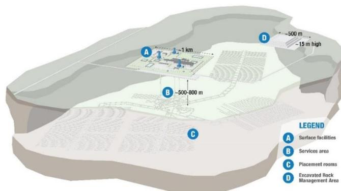
**Figure 1-2: Conceptual Design of Deep Geological Repository Site**
