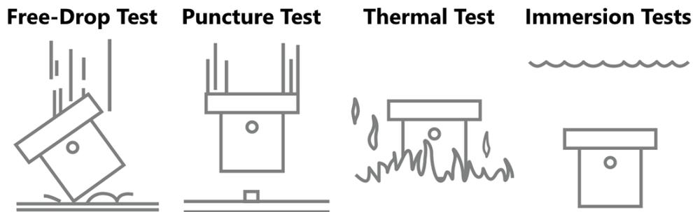
**Figure 5: Regulatory tests applicable to Type B packages**
