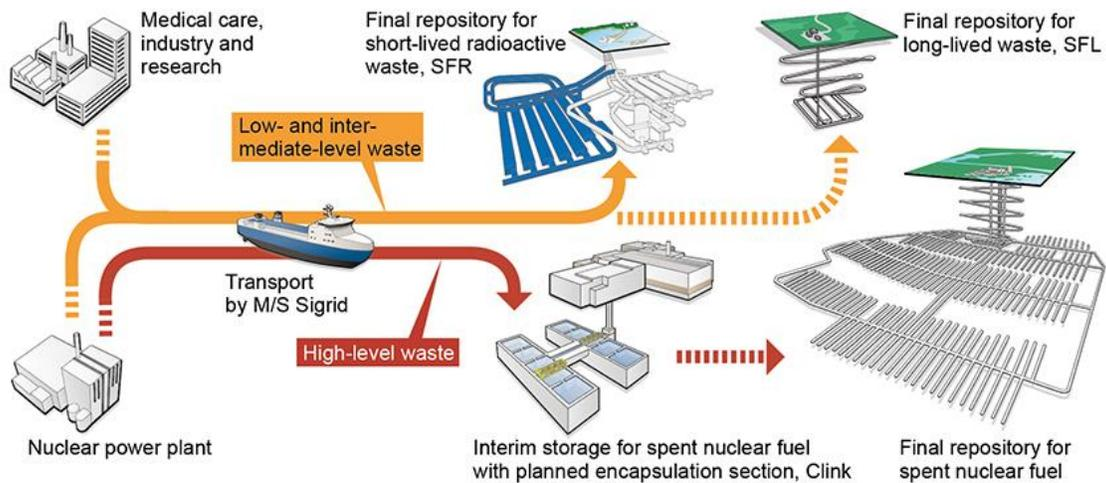
**Figure 7-3: Radioactive waste management and transportation system in Sweden [74]**
