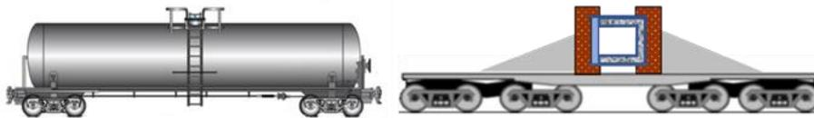
**Figure J-5: Tank railcar (left) and used fuel railcar (right) – note that the DSC-TP is shipped horizontally**
