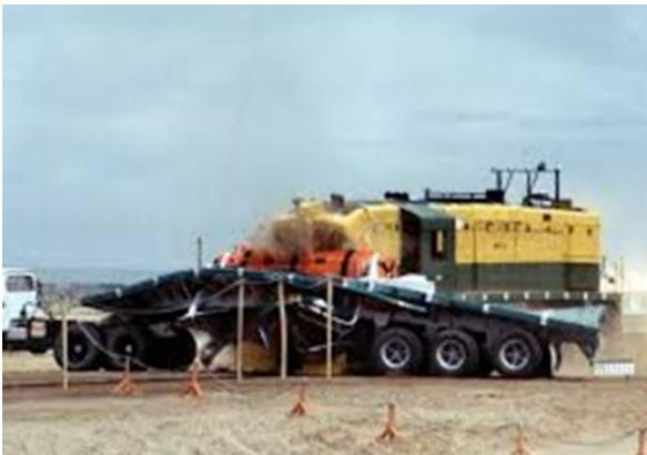
**Figure 4-2: Results of rail-truck collision**
