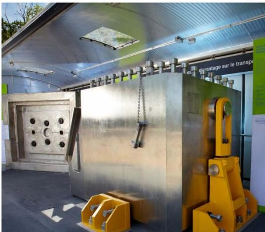
**Figure 2: Used Fuel Transportation Package (UFTP)**
